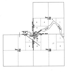
This plat represents the survey of an island in the Flint River, in secs. 28, 34, and 35, which was not included in the original survey of 7. 8 N., R. 5 E., as represented on the undated plat of the survey of 1822.
