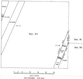
This plat represents the retracement and recessablishment of the boundaries of the 14,80 are tract of public land in sec. 24, as shown upon the plat approved May 29, 1850, in their true original positions according to the best available evidence of the position of the original corners.
