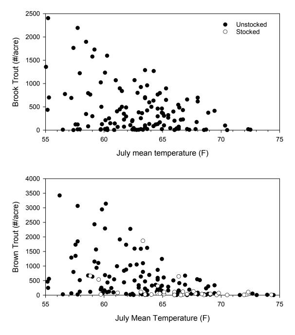
Figure 10.–Relationships between July mean water temperature and Brook and Brown trout density. Each dot represents observations from an individual stream location. The decline in the maximum trout density observed as stream temperatures increase indicates that the potential of a river reach for supporting trout decreases as stream conditions warm.
