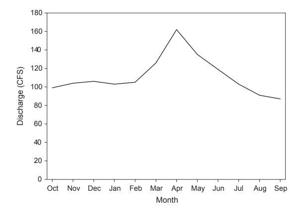
Figure 6.–Mean monthly discharge for the Boardman River for the period of record (1997–2005). Data are shown from October through September, a traditional water year. Source: United States Geological Survey, Ranch Rudolf gage station.
