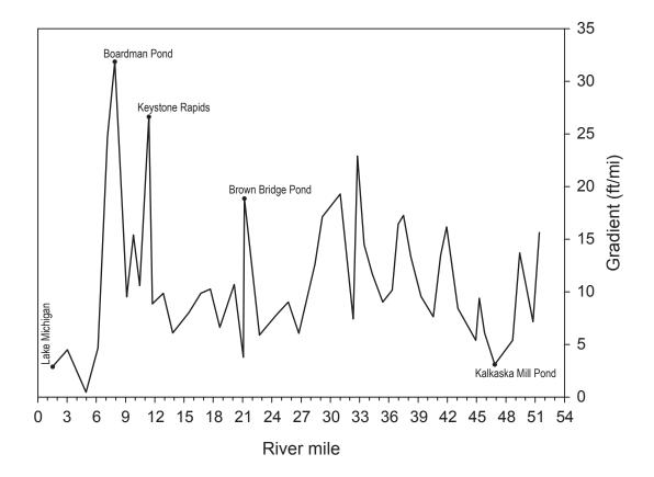
Figure 9.-Gradient (elevation change in feet per mile) of the Boardman River.
