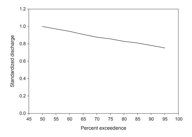
Figure 8.–Standardized low flow exceedence curves for the Boardman River (1997–2005). Standardized discharge is the discharge (Q)/ median (50% Q) discharge. Exceedence curves represent the probability of a discharge exceeding a given value. Source: United States Geological Survey Ranch Rudolf gage station.
