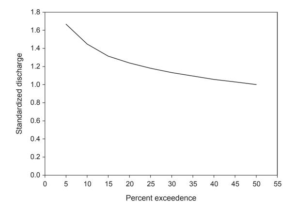
Figure 7.–Standardized high flow exceedence curves for the Boardman River (1997–2005). Standardized discharge is the discharge (Q)/ median (50% Q) discharge. Exceedence curves represent the probability of a discharge exceeding a given value. Source: United States Geological Survey, Ranch Rudolf gage station.
