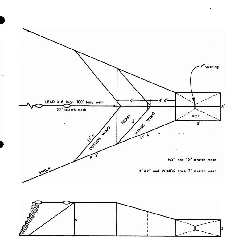
Figure III-2.--Construction details of a 6/3-foot trap net (6-foot lead tapering to a 3-foot pot).
