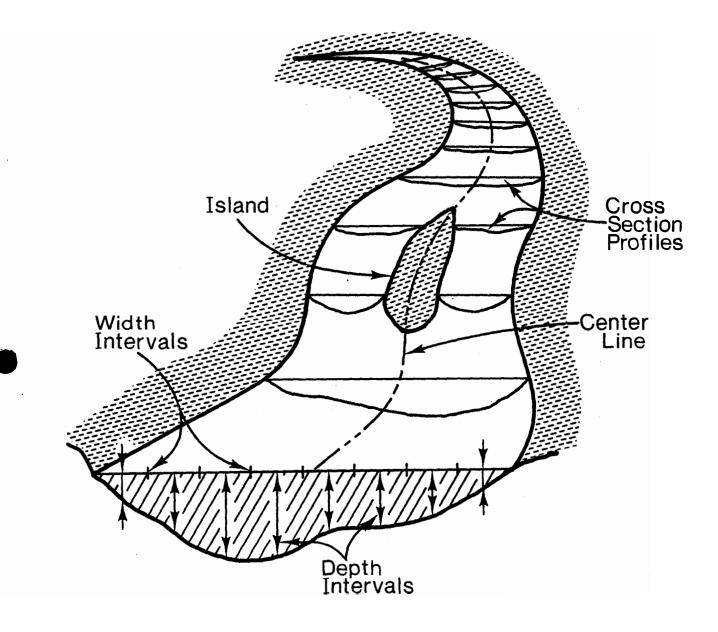
Figure II-3.--A stream sample station showing: morphology measurements of length, widths, depths, and cross-section profiles.
