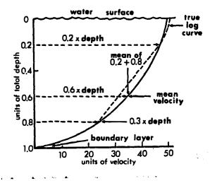
Figure 2. -- The rate of flow of water at different depths in an open channel, and depths at which the mean flow can be measured. (Taken from Hynes 1970)
