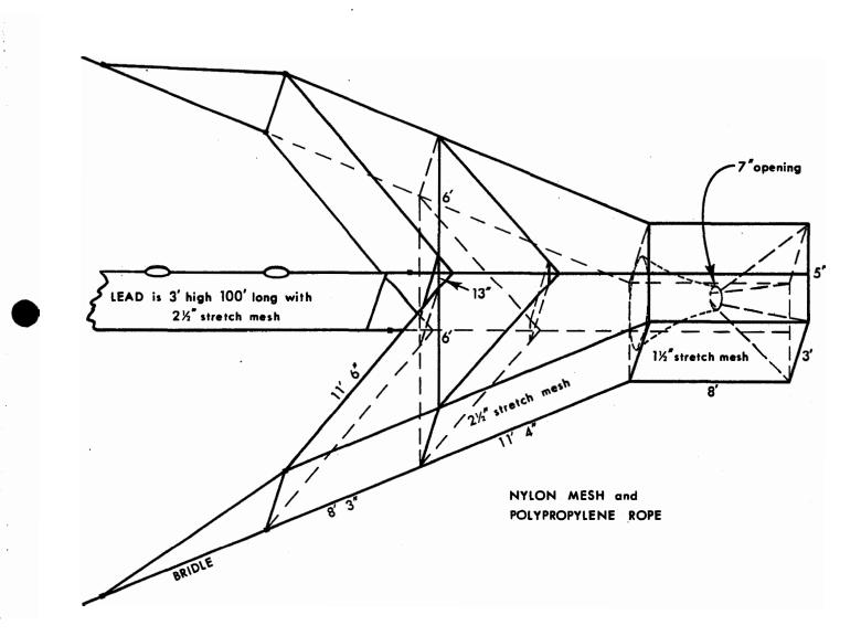
. Figure III-1. --Construction details of a 3-foot trap net.
