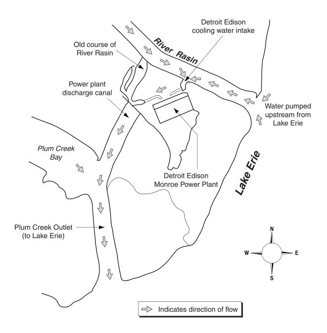
Figure 22.–Detroit Edison Monroe Power Plant cooling water flow configuration. Data from: aerial photograph, Engineering Department, City of Monroe.
