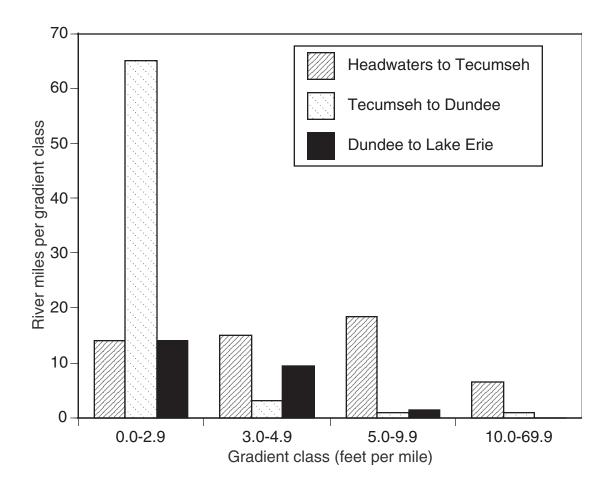
Figure 12.–Gradient classes and length of river in each for three sections of the River Raisin mainstem. Data from: P. Seelbach and G. Whelan, Michigan Department of Natural Resources, Fisheries Division, personal communication.
