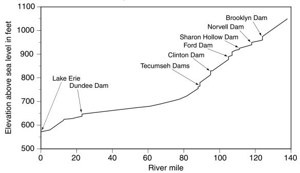
Figure 11b.–Elevation changes by river mile from the mouth to the headwaters of the River Raisin mainstem. Selected major dam locations are noted. Data from: Knutilla and Allen 1975.
