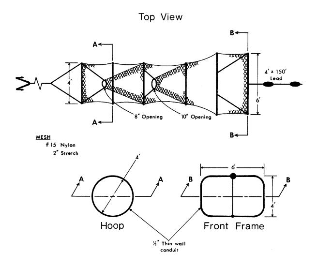
Figure 3.3–Construction details of a fyke net.
