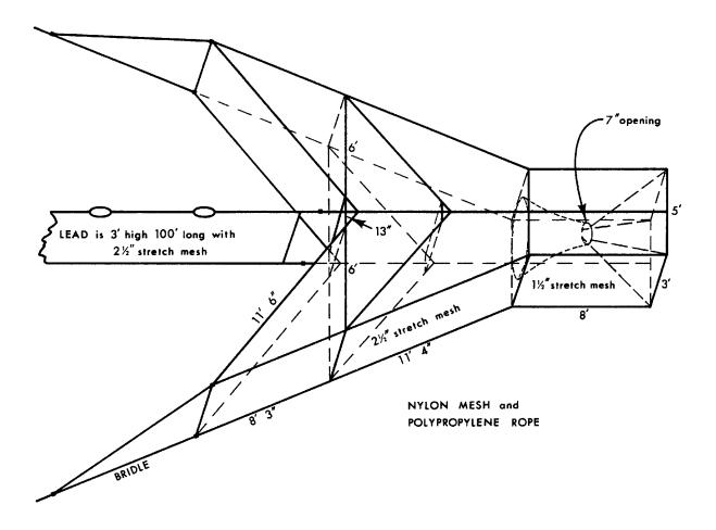
Figure 3.1–Construction details of a 3-foot trap net.
