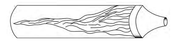
Figure 19.3–A rubber-bag current meter. (from Hynes 1970)
