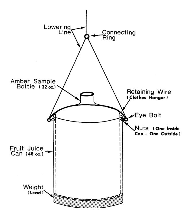
Figure 2.4–Phytoplankton (chlorophyll) sampler construction plans.
