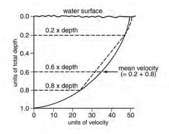
Figure 19.2–The rate of flow of water at different depths in an open channels, and depths at which the mean flow can be measured. (modified from Hynes 1970)
