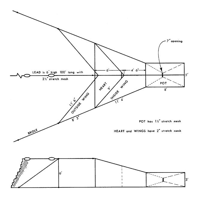
Figure 3.2–Construction details of a 6/3-foot trap net (6-foot lead tapering to a 3-foot pot).
