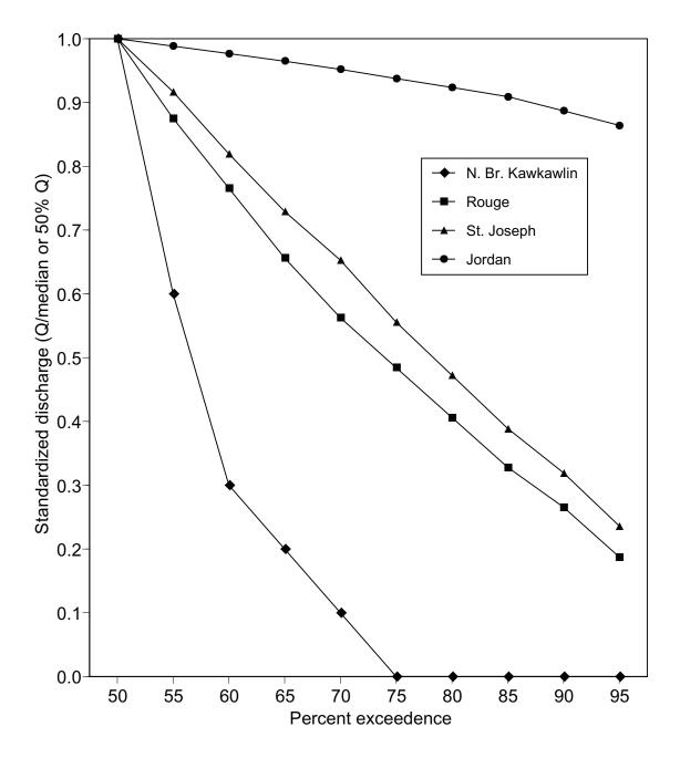
Figure 9.—Standardized low flow exceedence curves for four Michigan rivers. Standardized discharge is the discharge (Q) / median(50% Q) discharge. Exceedence curves represent the probability of a discharge being equaled or exceeded for a given value. Data from United States Geological Survey gauge stations for period of record.
