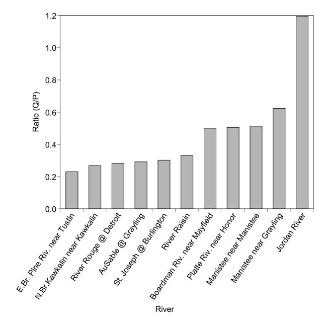
Figure 11.—Ratio of flow (Q) to precipitation (P) in the catchment basin for several rivers in Michigan. Flow expressed as inches of precipitation in the watershed. Data from United States Geological Survey, stream discharge records.
