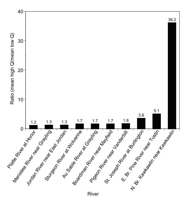
Figure 7.—Ratio of means of monthly streamflows (Q) for months with highest and lowest mean flows for period of record. Data are from United States Geological Survey, stream discharge records.
