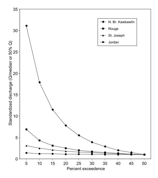
Figure 8.–Standardized high flow exceedence curves for four Michigan rivers. Standardized discharge is the discharge (Q) / median  $(50\% \, Q)$  discharge. Exceedence curves represent the probability of a discharge being equaled or exceeded for a given value. Data from United States Geological Survey gauge stations for period of record.
