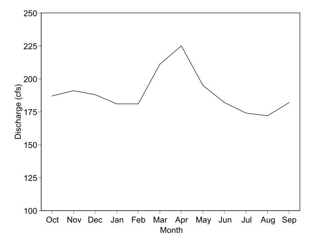
Figure 6.—Mean monthly discharge for Jordan River near East Jordan for period of record (1967-97). Data are shown from October through September, a traditional water year. Data are from United States Geological Survey, stream discharge records (gauge number 04127800).
