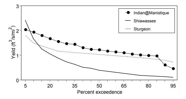
Figure 15.–Yield ( $ft^3/s/mi^2$ ) exceedence curves for the Tributaries–lower Indian River. Comparison exceedence curves are given for the Shiawassee and Sturgeon rivers. Exceedence curve represents the frequency of a discharge exceeding a given rate. Data from the United States Geological Service for period of record.
