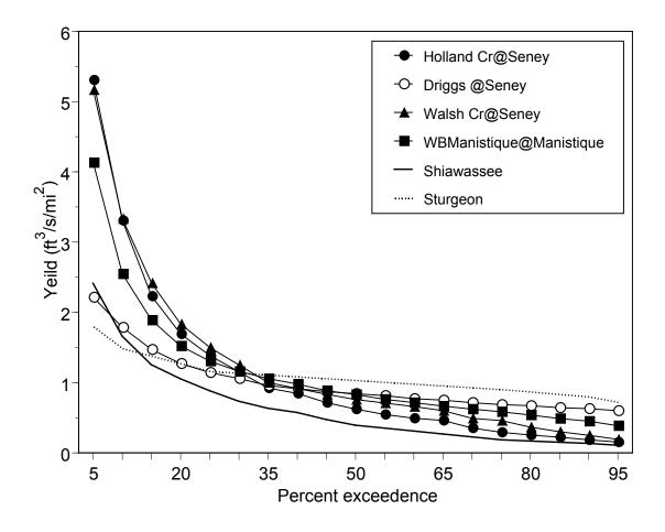
Figure 11.–Yield (ft<sup>3</sup>/s/mi<sup>2</sup>) exceedence curves for the Tributaries–central basin sites (4). Comparison exceedence curves are given for the Shiawassee and Sturgeon rivers. Exceedence curve represents the frequency of a discharge exceeding a given rate. Data from the United States Geological Service for period of record.
