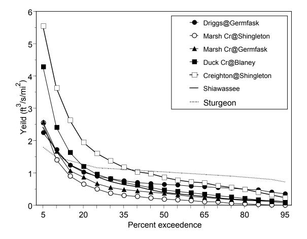
Figure 12.–Yield  $(ft^3/s/mi^2)$  exceedence curves for the Tributaries–central basin sites (5). Comparison exceedence curves are given for the Shiawassee and Sturgeon rivers. Exceedence curve represents the frequency of a discharge exceeding a given rate. Data from the United States Geological Service for period of record.
