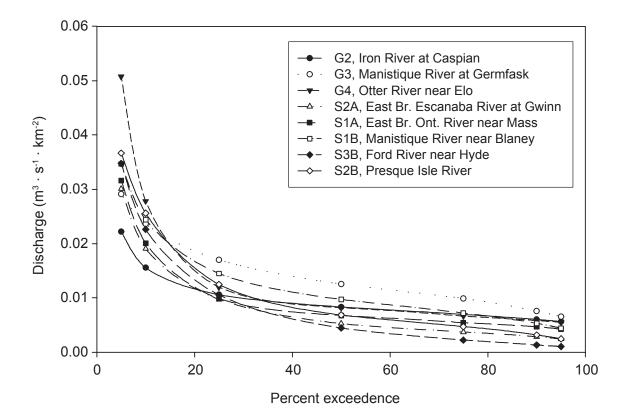
Figure 1.–Flow exceedence curves representing the range of stream-flow patterns present in Upper Peninsula rivers. Streams that are dominated by groundwater inputs have codes beginning with G and streams that are surface water dominated have codes beginning with S. See text for code definitions.
