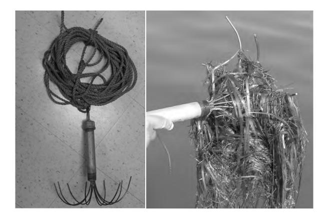
Figure 4.–Photographs of hook designed and constructed to sample submerged plants in Lake St. Clair. Hook was constructed from iron pipe filled with lead and armed with eight times of steel drill rod.
