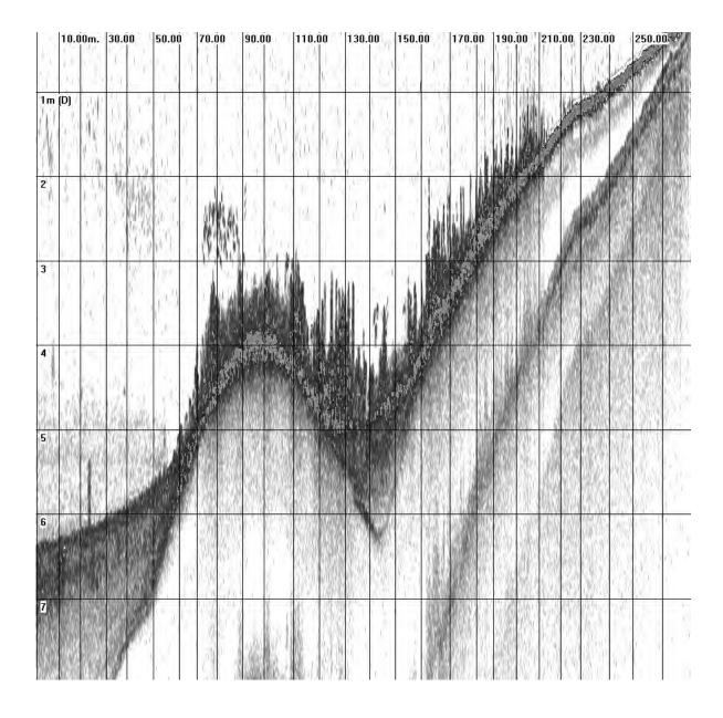
Figure 6.–Example echogram from hydroacoustic data file showing water depth, lake bottom, submerged plants, and school of fish. Plant analysis software extracts geographic position, water depth, plant height, and plant coverage from these hydroacoustic files.
