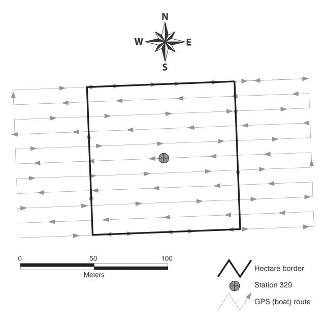
Figure 5.–Example map of hydroacoustic transects over one square hectare spaced 10 m apart and centered on station 329 in Lake St. Clair. Hydroacoustic data were post-processed and clipped to the hectare polygon. Hook tosses were generally made near the center unless plants were only observed near an edge of the square hectare.
