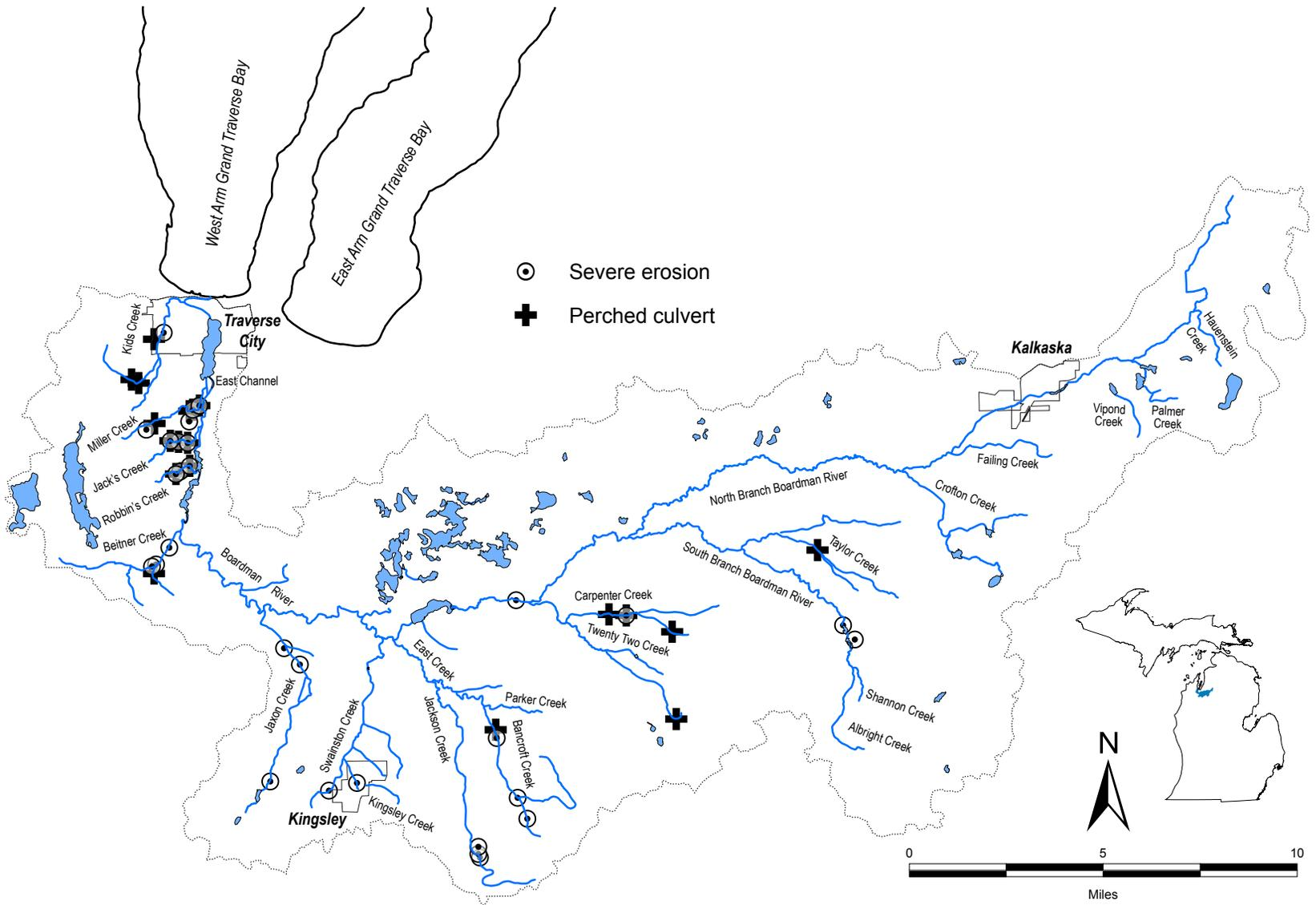
Figure 14.—Severe erosion and perched culvert sites within the Boardman River watershed.
