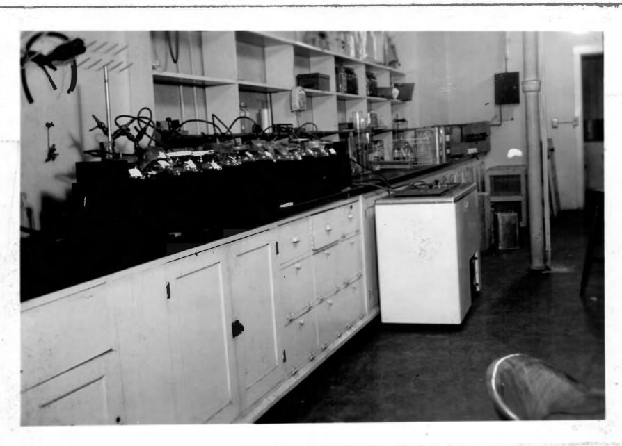
Figure 1.--View of laboratory equipment used in BDT toxicity tests, showing temperature control unit and arrangement of test jars.
