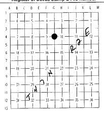
A. Description of original monument and accessories and/or subsequent restoration: (G-4) 1/4 Corner common to Sections 9 and 10. Township 47 North, Range 2 East. John Mullett set the original 1/4 section post in 1845. County surveyor records from the 1920's describe the corner as a 1" x 36" bolt with two Maples for witnesses. In 1981 W.L. Karr found one bearing tree and one stump as described in REVA CO recorded in Liber 5 at Page 074 of the Chippewa County Corner Records.
