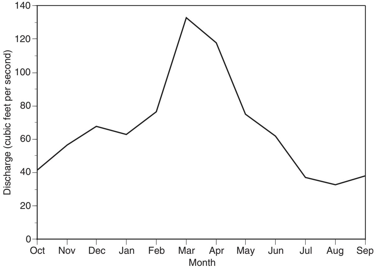
Figure 7.—Mean monthly discharge (cfs) for Rouge River in Southfield for period of record (1958-94). Data from: United States Geological Survey.
