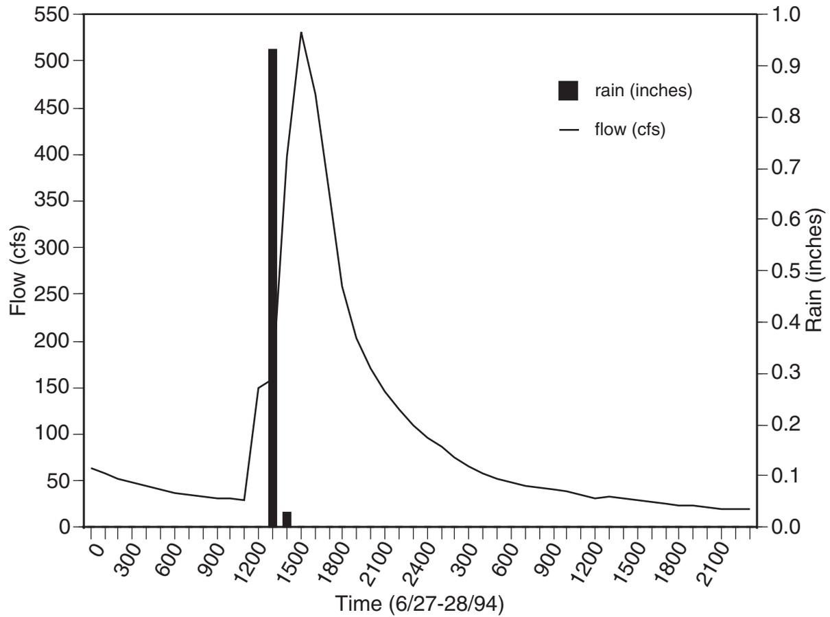
Figure 22.—Middle Rouge River (in Novi) flow in response to 6/26/94 rain event. Data from: Rouge Program Office. Depicts almost immediate response to rain event with rapid recovery. Indicates presence of impervious surfaces and storm sewers. Rain is expressed as an hourly average.
