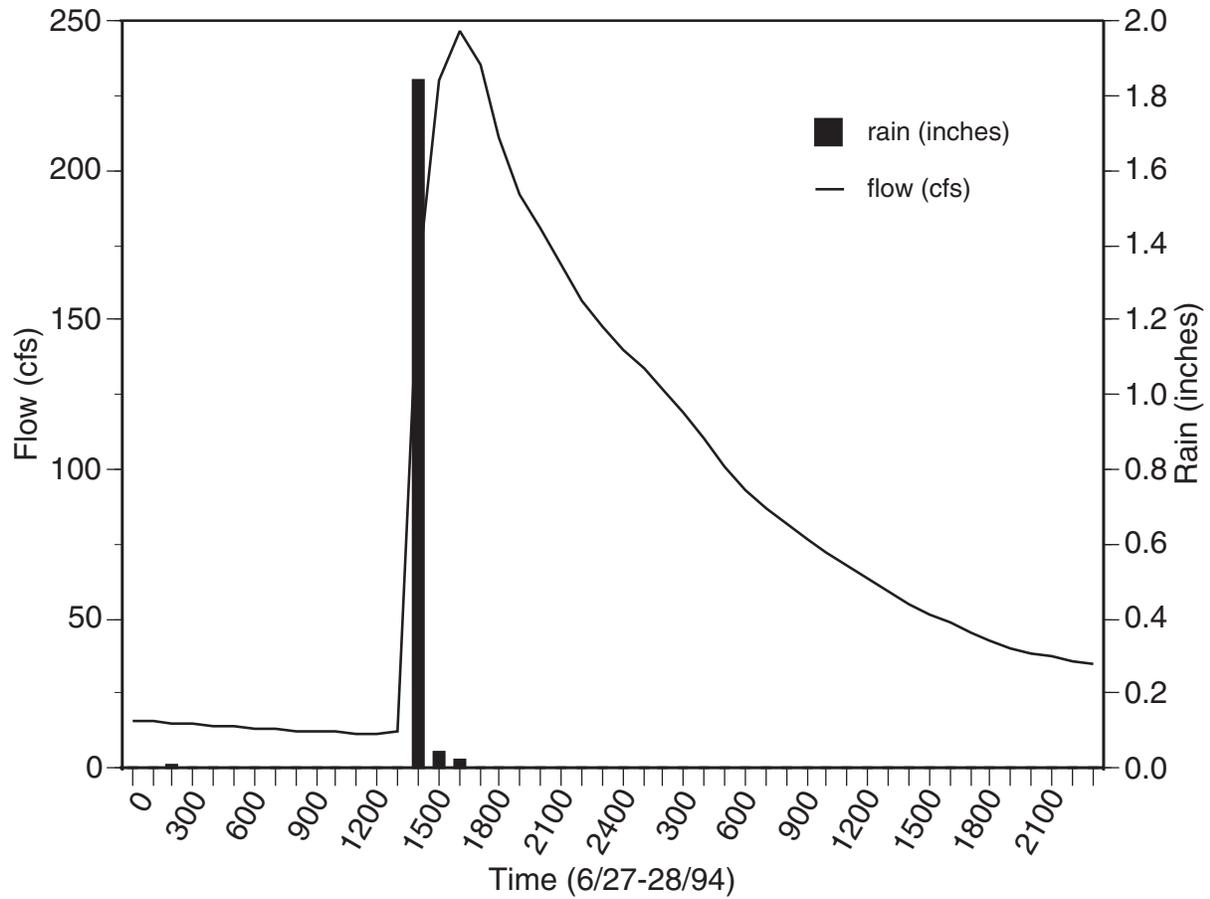
Figure 20.—Mainstem (in Bloomfield Hills) flow in response to 6/27/94 rain event. Data from: Rouge Program Office. Depicts almost immediate response to rain event with rapid recovery. Indicates presence of impervious surfaces, combined sewer overflows, and storm sewers. Rain is expressed as an hourly average.
