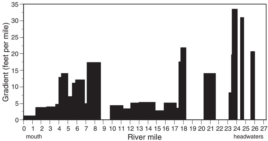
Figure 28a.—Gradient (elevation change in feet per mile) of the Middle Rouge River. Values are of stream bottom in tenths of river mile. Gradient is shown without existing dams or lake-level control structures. Data from: United States Geological Survey topographic maps.
