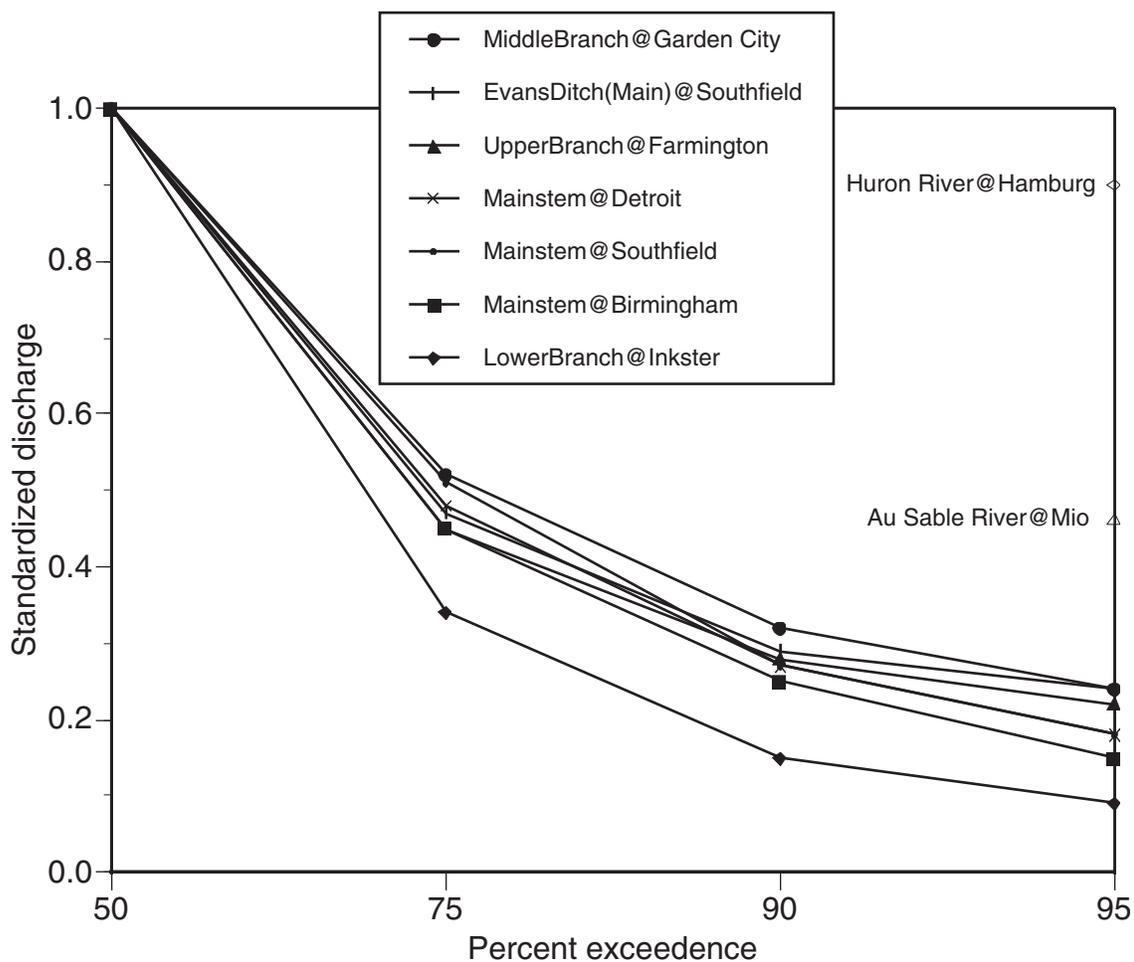
Figure 19.—Standardized low flow exceedence curves for three main branches and mainstem of Rouge River and Evans Ditch. Information from United States Geological Survey gauge stations for period of record. Standardized discharge is discharge/median (50%) discharge. Shown for comparison are neighboring Huron River and extremely stable, groundwater fed Au Sable River.
