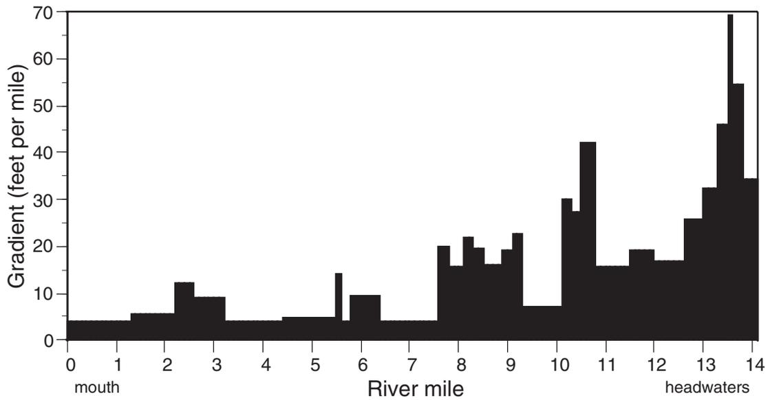
Figure 27a.—Gradient (elevation change in feet per mile) of the Upper Rouge River. Values are of stream bottom in tenths of river mile. Gradient is shown without existing dams or lake-level control structures. Data from: United States Geological Survey topographic maps.
