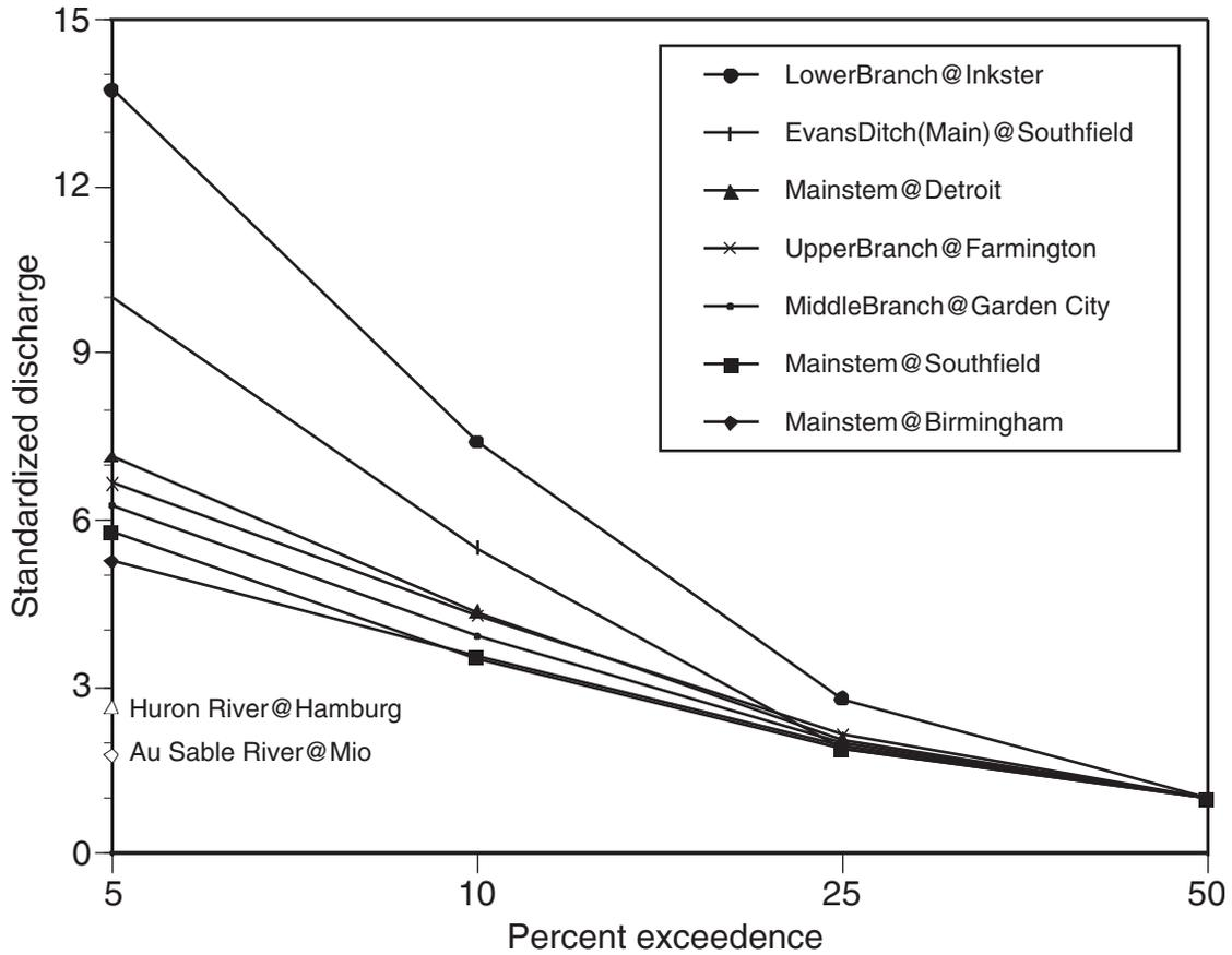
Figure 18.—Standardized high flow exceedence curves for three main branches and mainstem of Rouge River and Evans Ditch. Information from United States Geological Survey gauge stations for period of record. Standardized discharge is discharge/median (50%) discharge. Shown for comparison are neighboring Huron River and extremely stable, groundwater fed Au Sable River.
