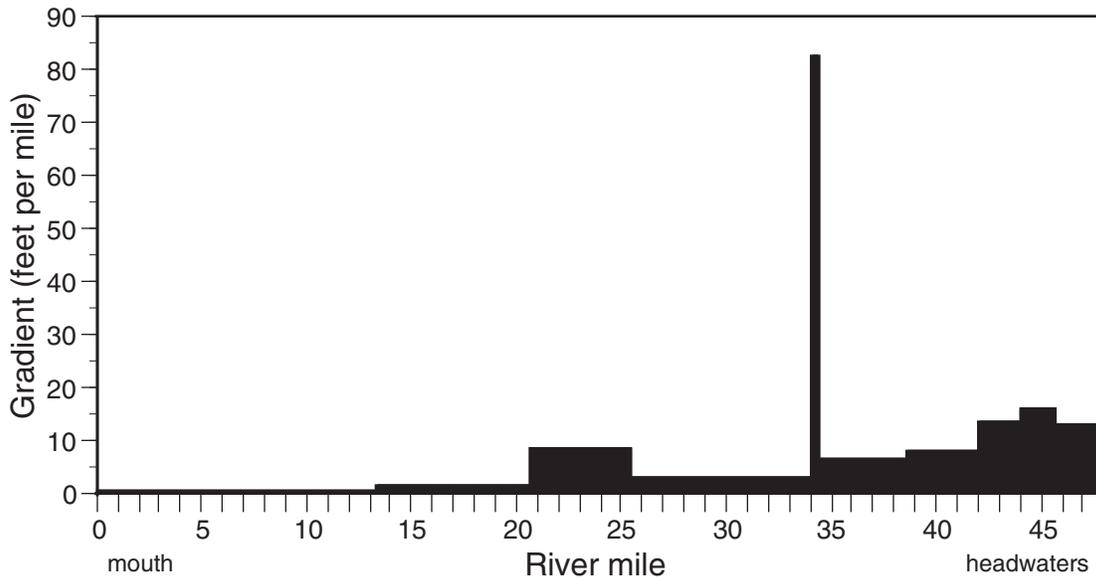
Figure 26a.—Gradient (elevation change in feet per mile) of the mainstem. Values are of stream bottom in tenths of river mile. Gradient is shown without existing dams or lake-level control structures. Data from: United States Geological Survey topographic maps.
