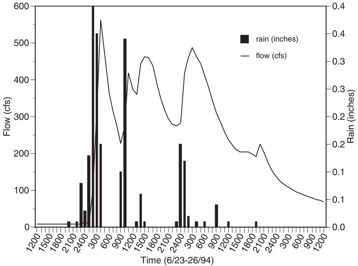
Figure 23.—Lower Rouge River (in Dearborn) flow in response to 6/23-26/94 rain events. Data from: Rouge Program Office. Depicts almost immediate response to rain event with rapid recovery. Indicates presence of impervious surfaces, combined sewer overflows, and storm sewers. Rain is expressed as an hourly average.
