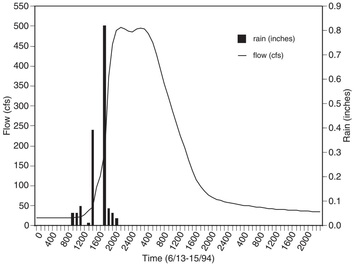
Figure 21.—Upper Rouge River (in Redford) flow in response to 6/13/94 rain event. Data from: Rouge Program Office. Depicts almost immediate response to rain event with rapid recovery. Indicates presence of impervious surfaces, combined sewer overflows, and storm sewers. Rain is expressed as an hourly average.
