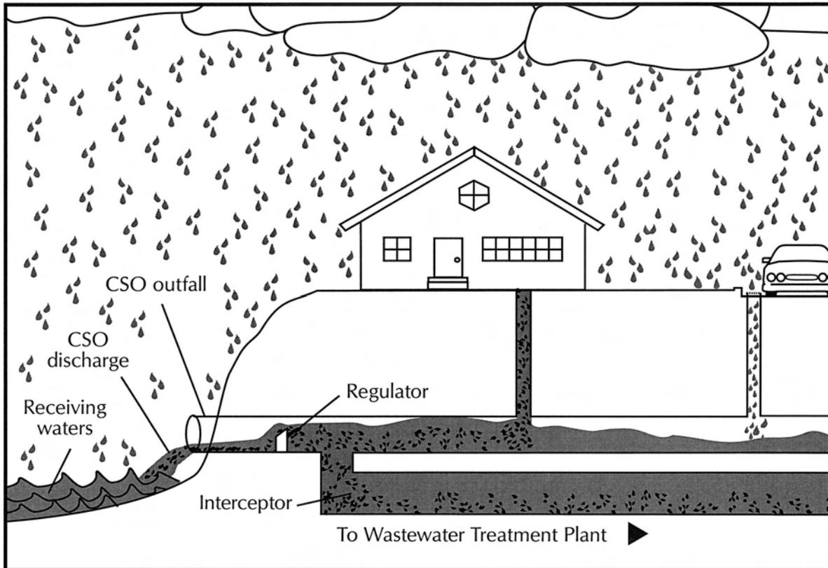
Figure 32.—Illustration of a typical combined sewer system. CSO = combined sewer overflow. Prepared by: Southeast Michigan Council of Governments.
