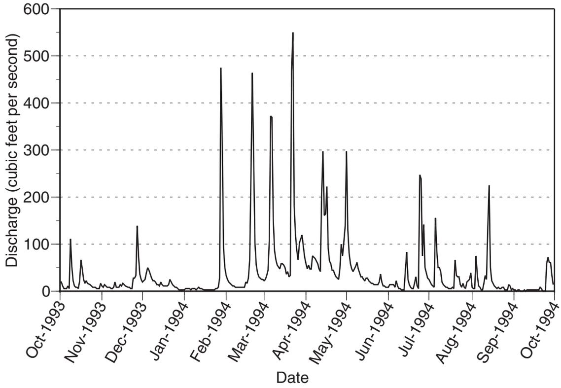
Figure 15.—Mean daily discharge of Lower River in Inkster for water year 1994. Data from: United States Geological Survey.
