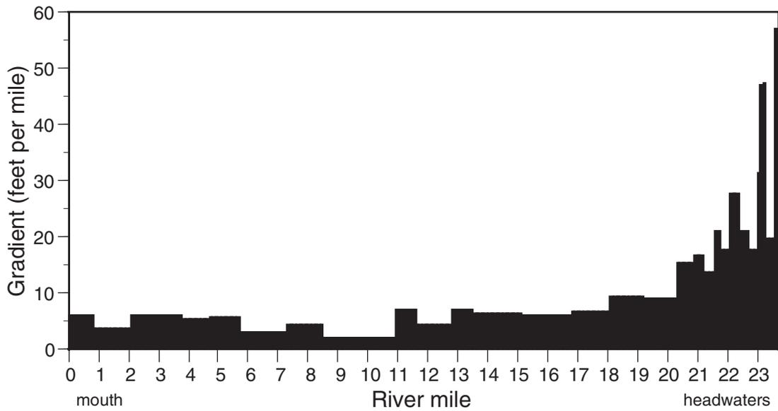
Figure 29a.—Gradient (elevation change in feet per mile) of the Lower Rouge River. Values are of stream bottom in tenths of river mile. Gradient is shown without existing dams or lake-level control structures. Data from: United States Geological Survey topographic maps.
