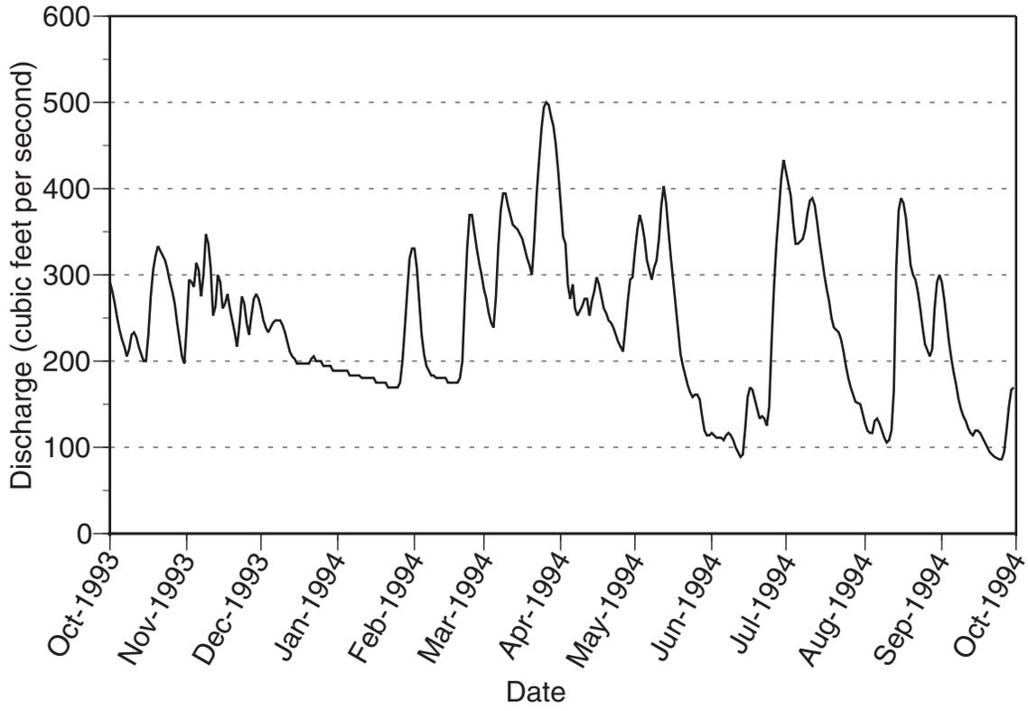
Figure 17.—Mean daily discharge of Huron River near Hamburg for water year 1994. Data from: United States Geological Survey.
