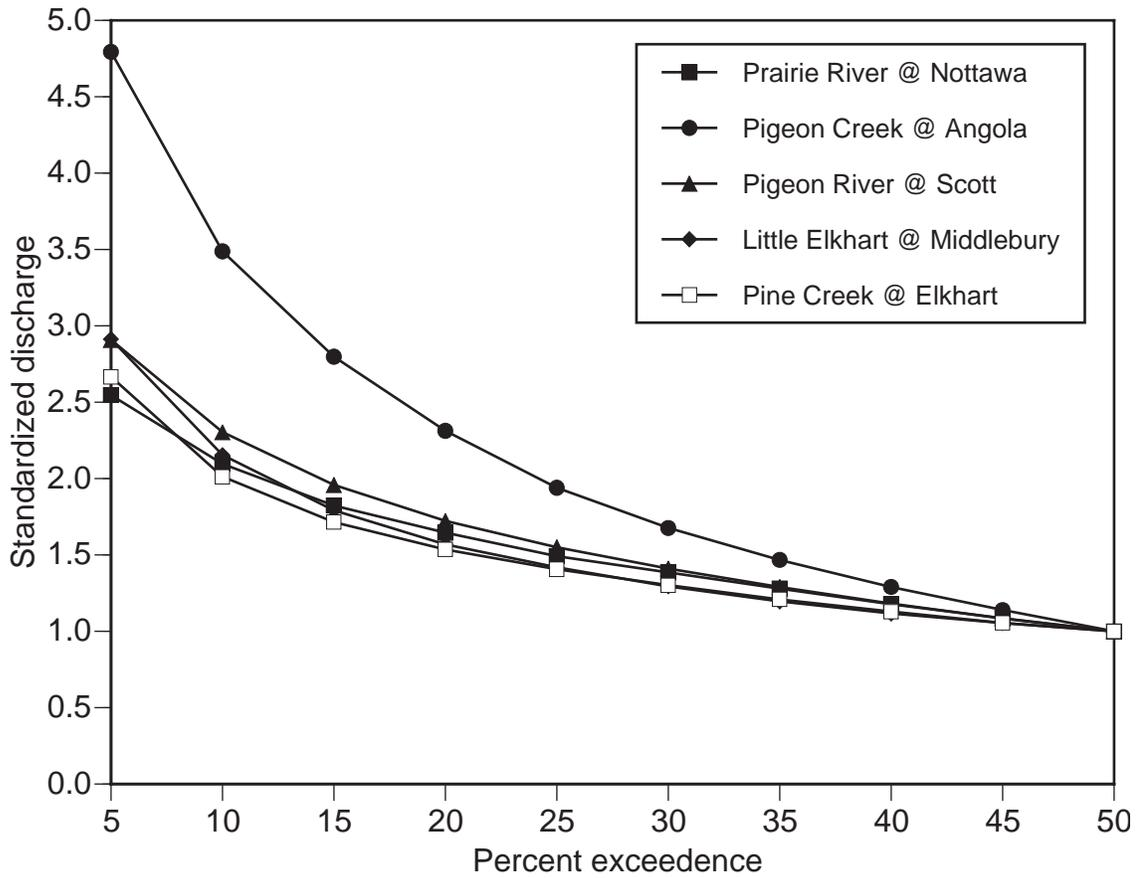
Figure 10.—Standardized high flow exceedence curves for major tributaries within the middle valley segment of St. Joseph River. Standardized discharge is the discharge (Q)/ median (50% Q) discharge. Exceedence curves represent the probability of a discharge exceeding a given value. Data from United States Geological Survey gauge stations for period of record.
