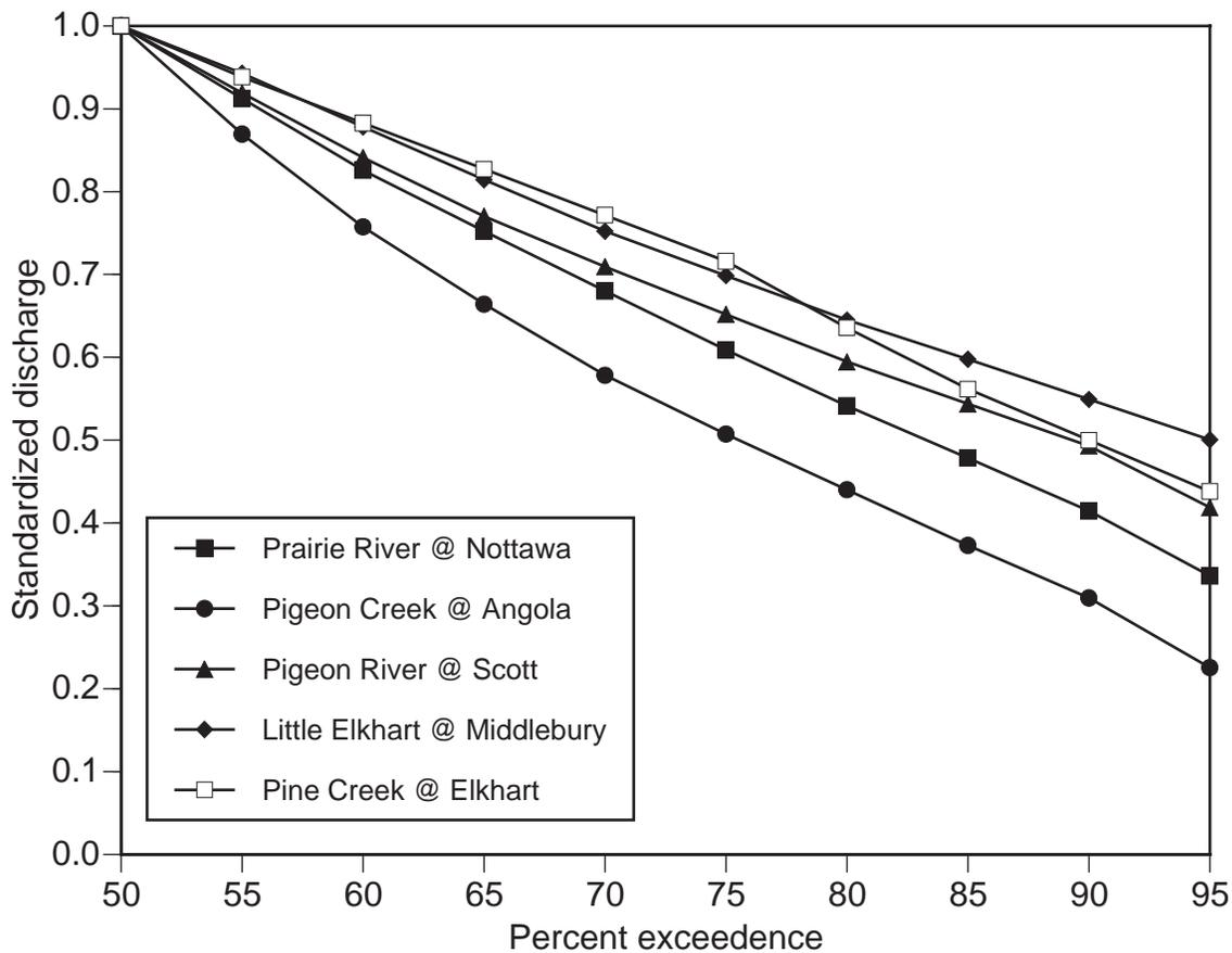
Figure 11.—Standardized low flow exceedence curves for major tributaries within the middle valley segment of St. Joseph River. Standardized discharge is the discharge (Q)/ median (50% Q) discharge. Exceedence curves represent the probability of a discharge exceeding a given value. Data from United States Geological Survey gauge stations for period of record.
