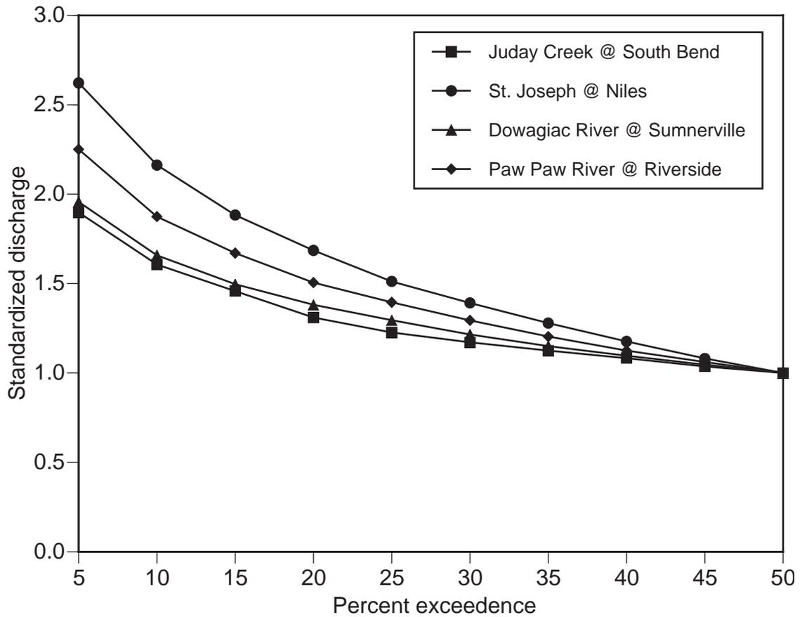
Figure 14.—Standardized high flow exceedence curves for mainstem and major tributaries within lower and mouth valley segments of St. Joseph River. Standardized discharge is the discharge (Q)/median (50% Q) discharge. Exceedence curves represent the probability of a discharge exceeding a given value. Data from United States Geological Survey gauge stations for period of record.
