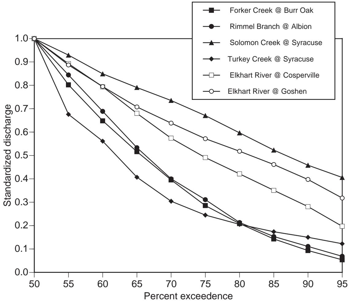
Figure 13.—Standardized low flow exceedence curves for Elkhart River and major tributaries. Standardized discharge is the discharge (Q)/ median (50% Q) discharge. Exceedence curves represent the probability of a discharge exceeding a given value. Data from United States Geological Survey gauge stations for period of record.
