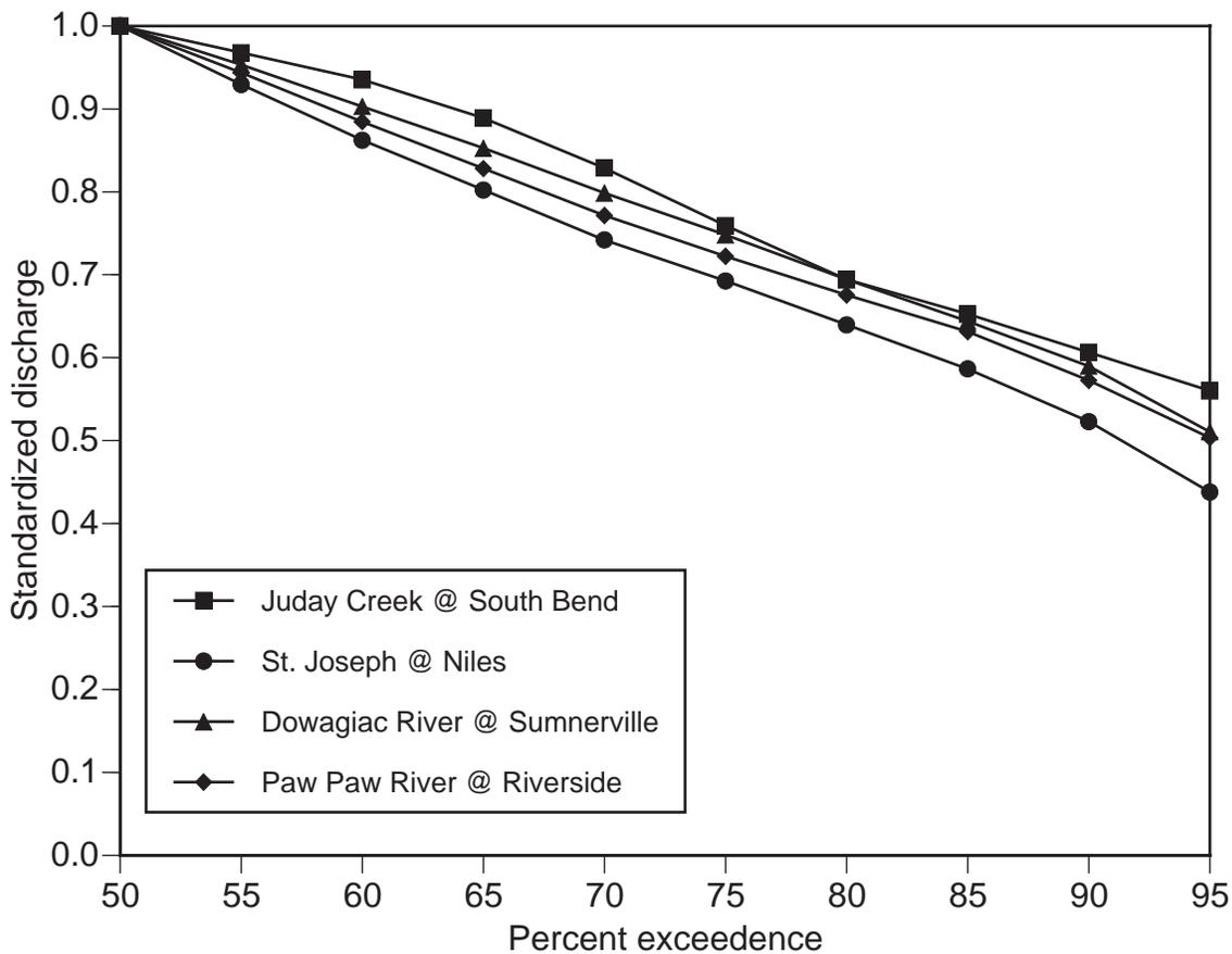
Figure 15.—Standardized low flow exceedence curves for mainstem and major tributaries within lower and mouth valley segments of St. Joseph River. Standardized discharge is the discharge (Q)/median (50% Q) discharge. Exceedence curves represent the probability of a discharge exceeding a given value. Data from United States Geological Survey gauge stations for period of record.
