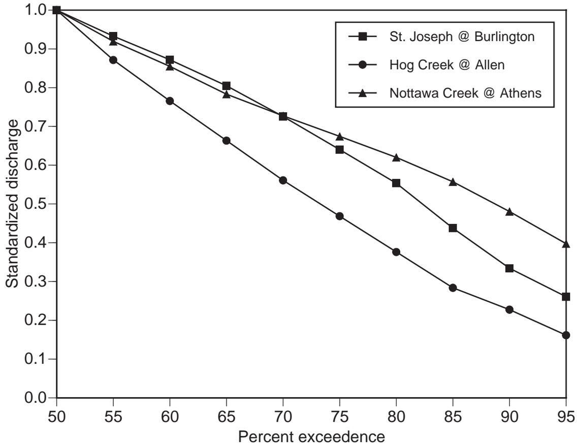
Figure 7.—Standardized low flow exceedence curves for St. Joseph River and tributaries in headwaters and upper valley segments. Standardized discharge is the discharge (Q)/ median (50% Q) discharge. Exceedence curves represent the probability of a discharge exceeding a given value. Data from United States Geological Survey gauge stations for period of record.
