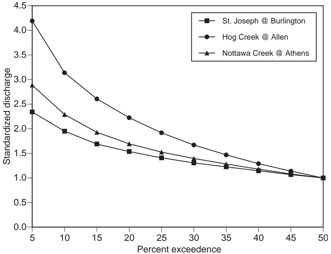
Figure 6.—Standardized high flow exceedence curves for St. Joseph River and tributaries in the headwaters and upper valley segments. Standardized discharge is the discharge (Q)/ median (50% Q) discharge. Exceedence curves represent the probability of a discharge exceeding a given value. Data from United States Geological Survey gauge stations for period of record.
