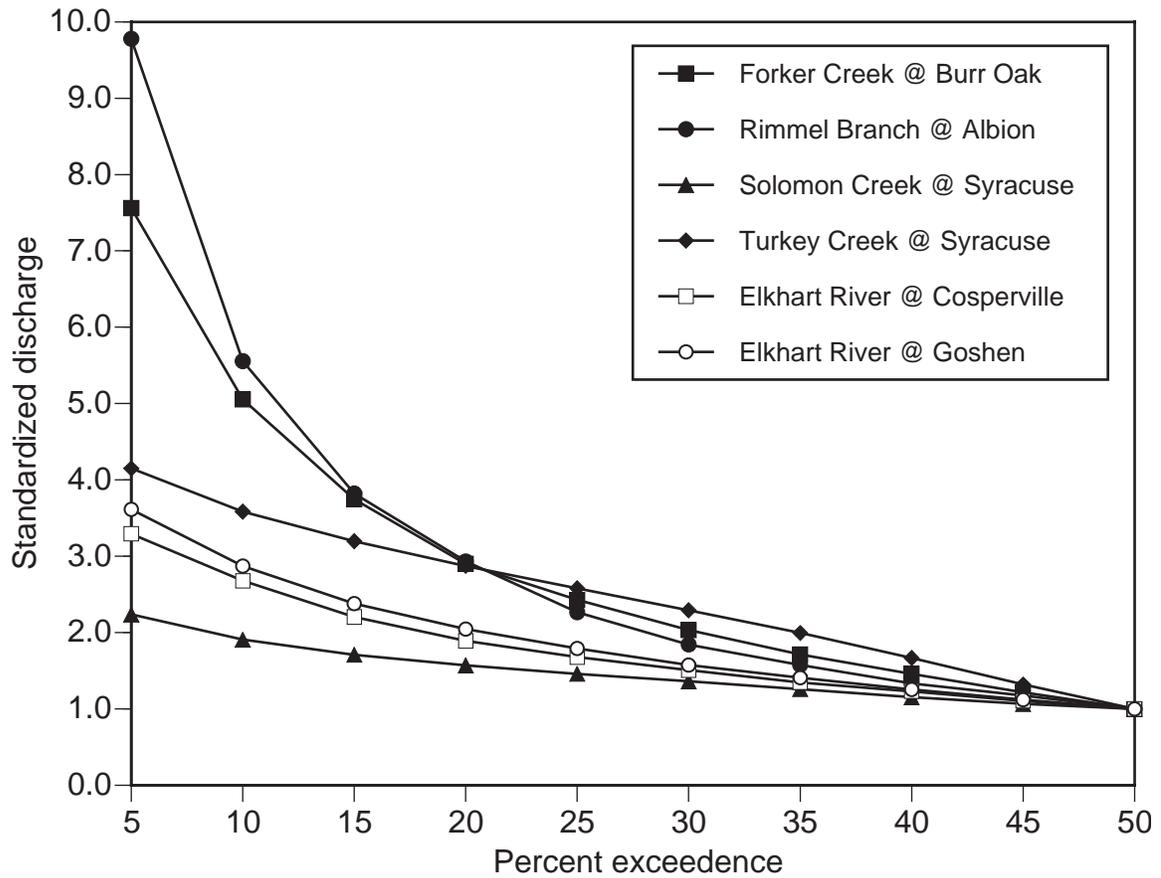
Figure 12.—Standardized high flow exceedence curves for Elkhart River and major tributaries. Standardized discharge is the discharge (Q)/ median (50% Q) discharge. Exceedence curves represent the probability of a discharge exceeding a given value. Data from United States Geological Survey gauge stations for period of record.
