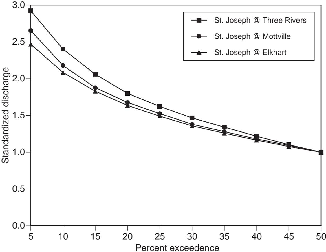
Figure 8.—Standardized high flow exceedence curves for mainstem of St. Joseph River within the middle valley segment. Standardized discharge is the discharge (Q)/ median (50% Q) discharge. Exceedence curves represent the probability of a discharge exceeding a given value. Data from United States Geological Survey gauge stations for period of record.
