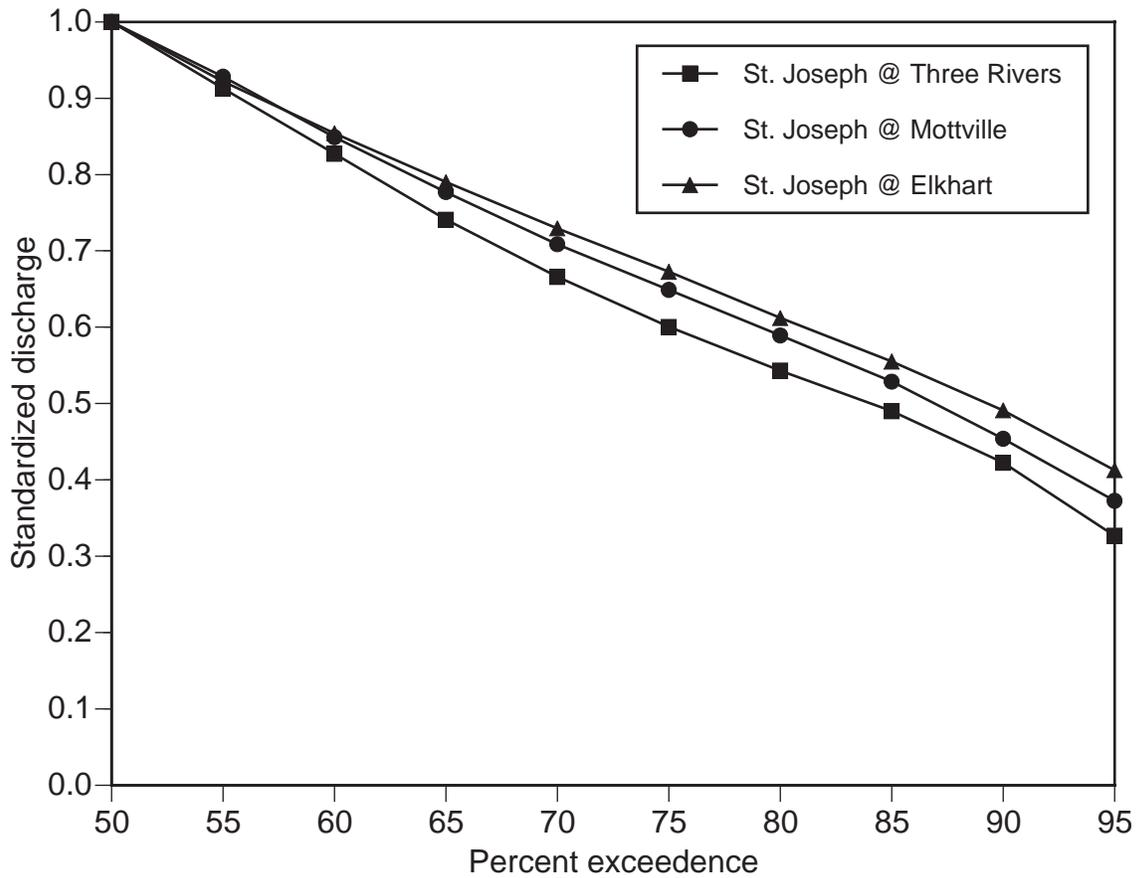
Figure 9.—Standardized low flow exceedence curves for mainstem of St. Joseph River within the middle valley segment. Standardized discharge is the discharge (Q)/ median (50% Q) discharge. Exceedence curves represent the probability of a discharge exceeding a given value. Data from United States Geological Survey gauge stations for period of record.
