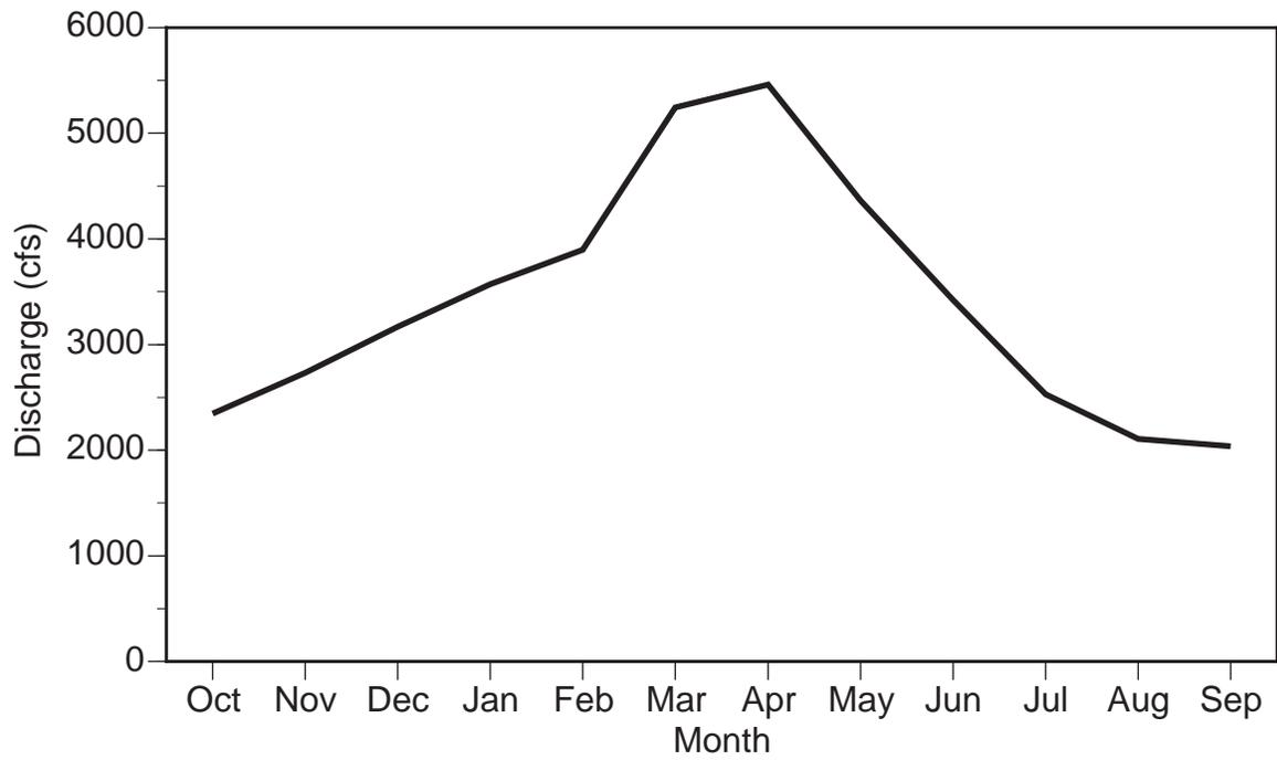
Figure 5.—Mean monthly discharge for St. Joseph River at Niles for period of record (1931-95). Data are shown from October through September, a traditional water year. Data from United States Geological Survey.
