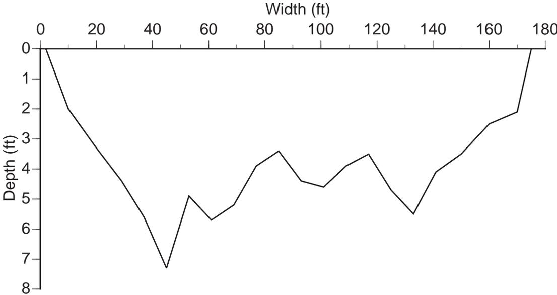
Figure 24a.—Stream channel cross-section of St. Joseph River at Three Rivers. Data from United States Geological Survey.
