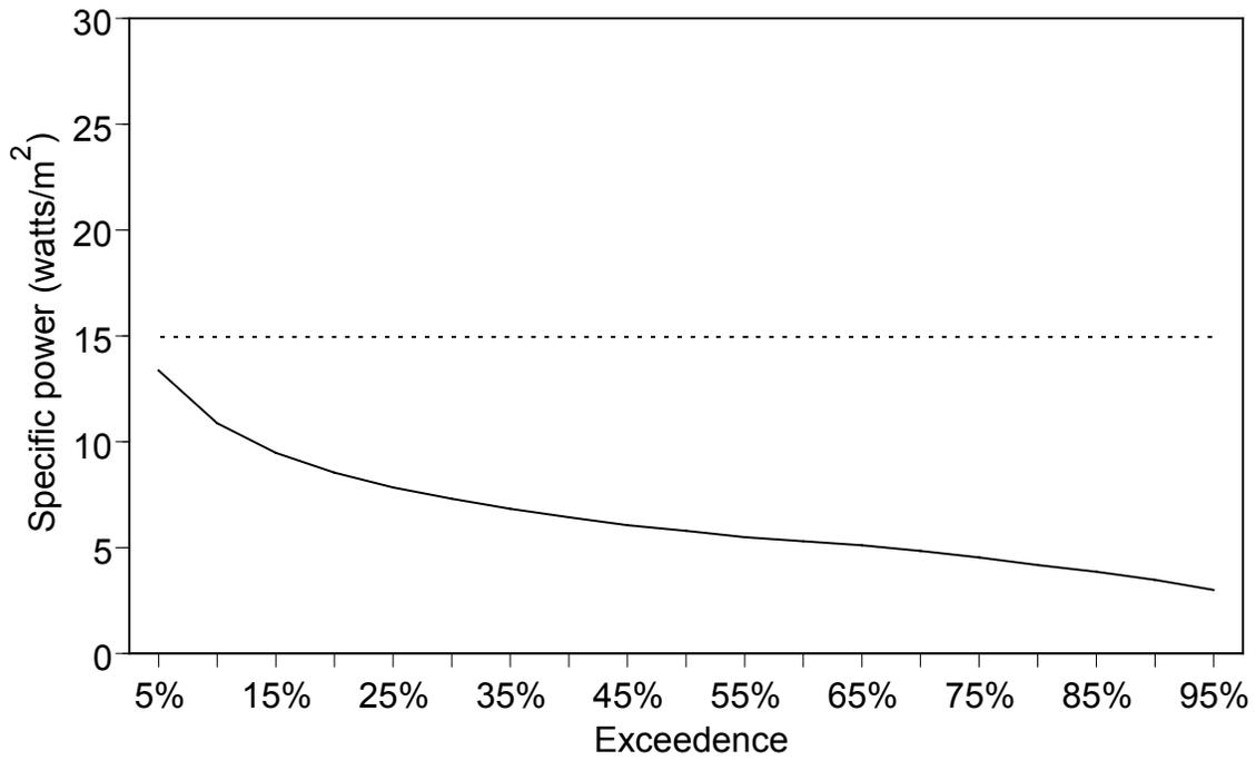
Figure 21.—Specific power for Manistique River at Germfask.
