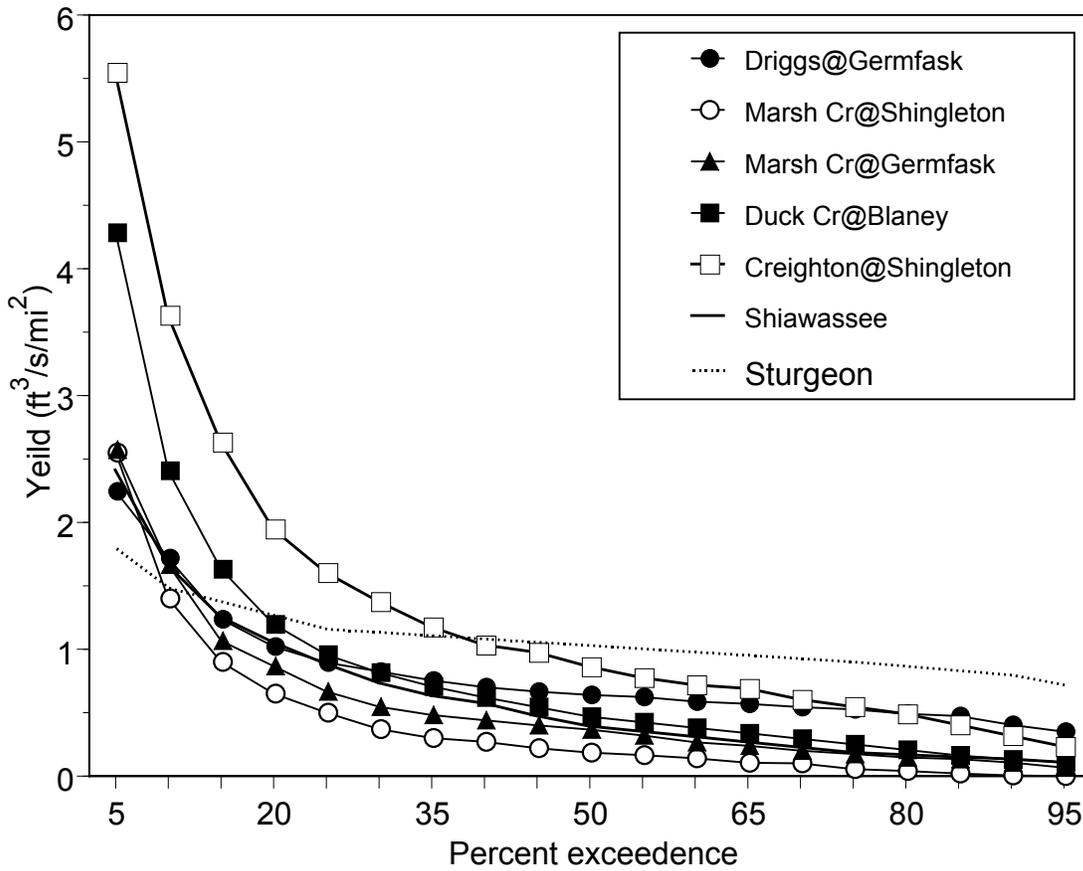
Figure 12.—Yield (ft³/s/mi²) exceedence curves for the Tributaries—central basin sites (5). Comparison exceedence curves are given for the Shiawassee and Sturgeon rivers. Exceedence curve represents the frequency of a discharge exceeding a given rate. Data from the United States Geological Service for period of record.
