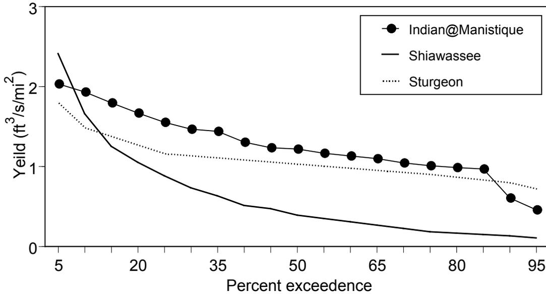
Figure 15.—Yield ( $\text{ft}^3/\text{s}/\text{mi}^2$ ) exceedence curves for the Tributaries—lower Indian River. Comparison exceedence curves are given for the Shiawasse and Sturgeon rivers. Exceedence curve represents the frequency of a discharge exceeding a given rate. Data from the United States Geological Service for period of record.
