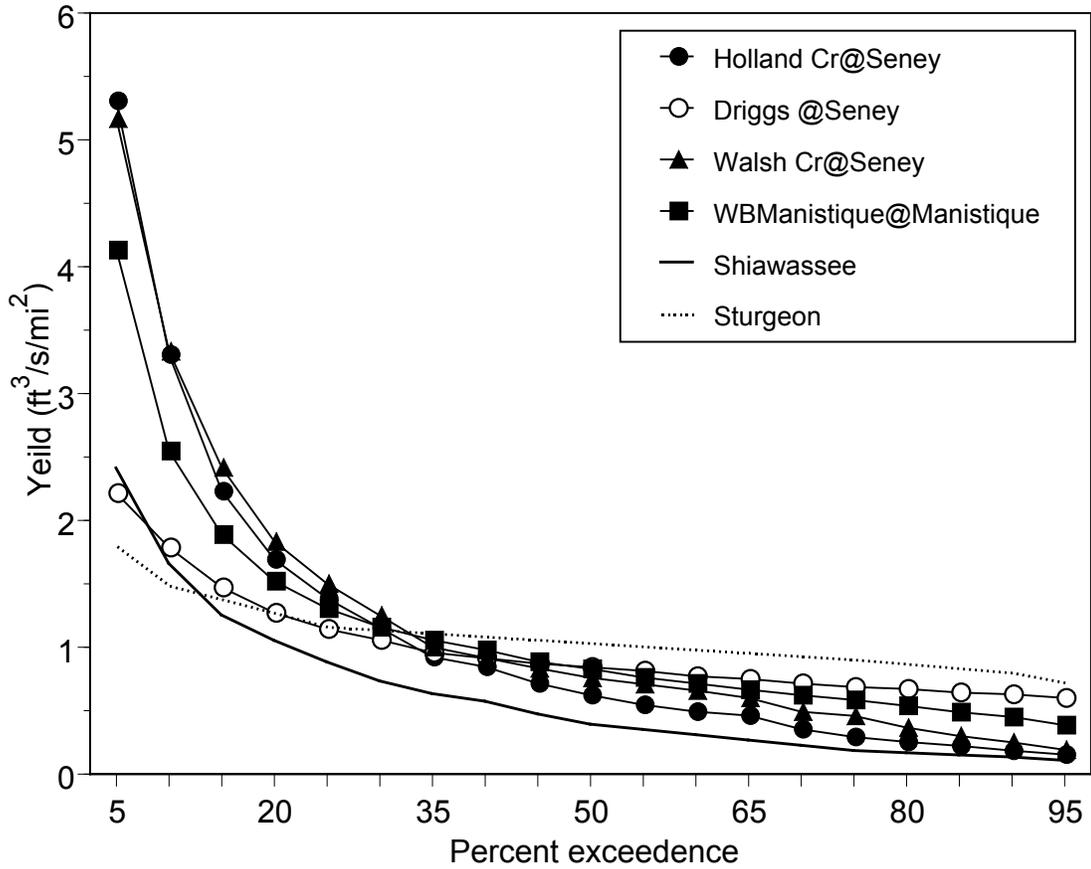
Figure 11.—Yield (ft<sup>3</sup>/s/mi<sup>2</sup>) exceedence curves for the Tributaries—central basin sites (4). Comparison exceedence curves are given for the Shiawassee and Sturgeon rivers. Exceedence curve represents the frequency of a discharge exceeding a given rate. Data from the United States Geological Service for period of record.
