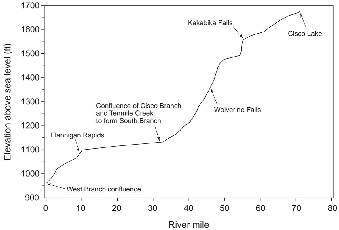
Figure 32.—Elevation changes by river mile for the Cisco Branch and South Branch Ontonagon rivers.
