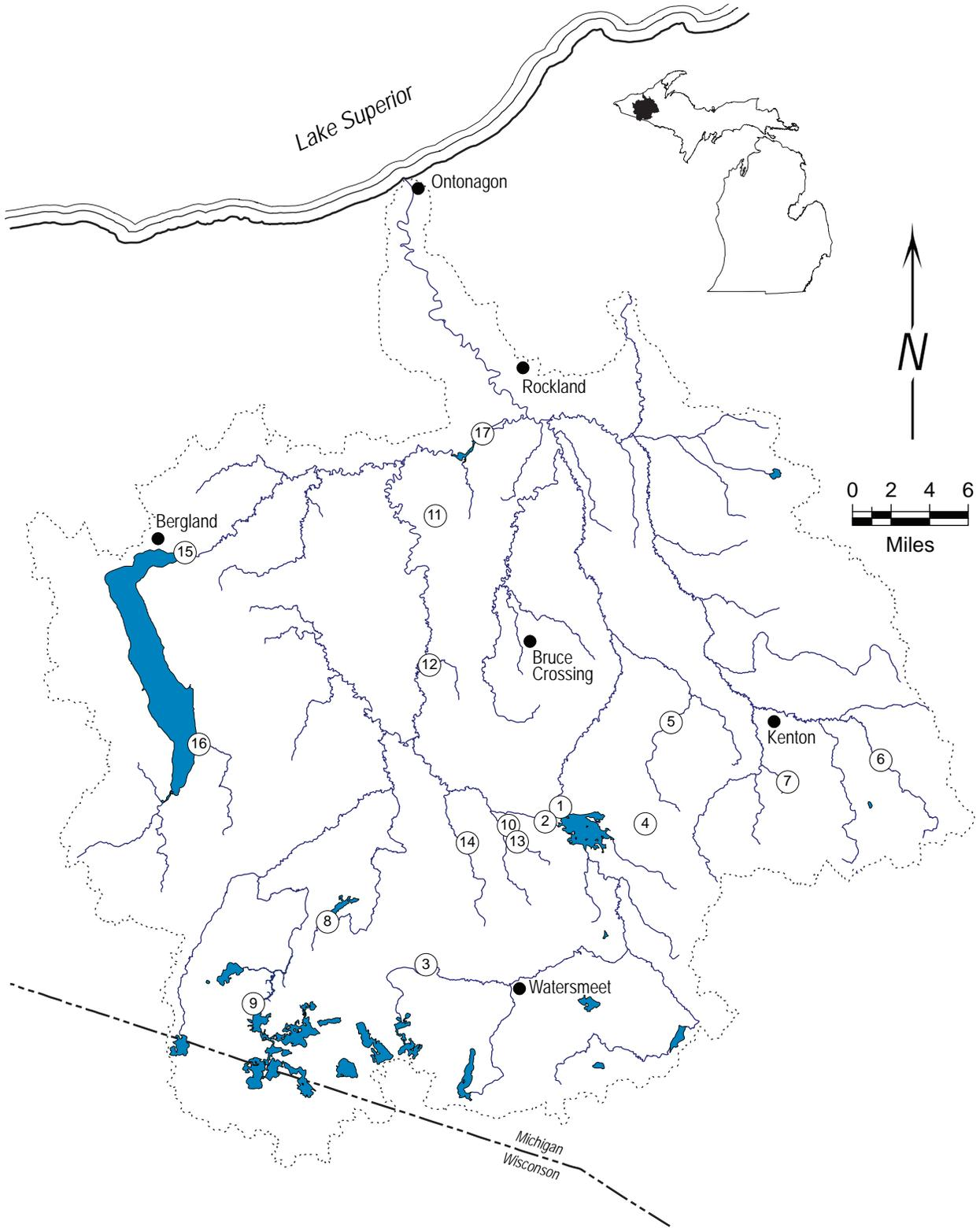
Figure 40.—Registered dams in the Ontonagon River watershed. (See Table 11 for dam descriptions.)
