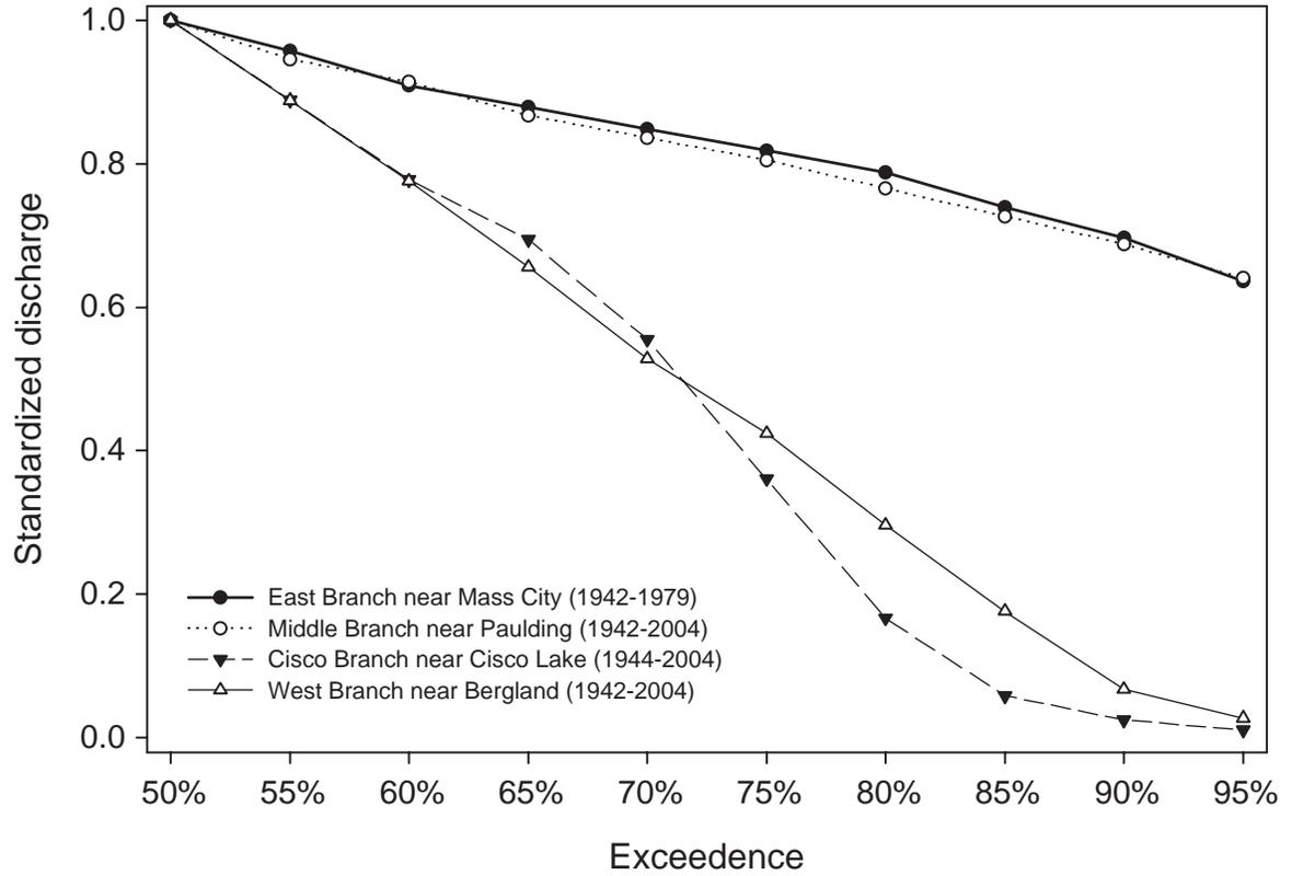
Figure 11.—Standardized low-flow duration curves for sites in the Ontonagon River watershed that are not affected by the Bond Falls diversion. Data from United States Geological Survey gauge stations for period of record.
