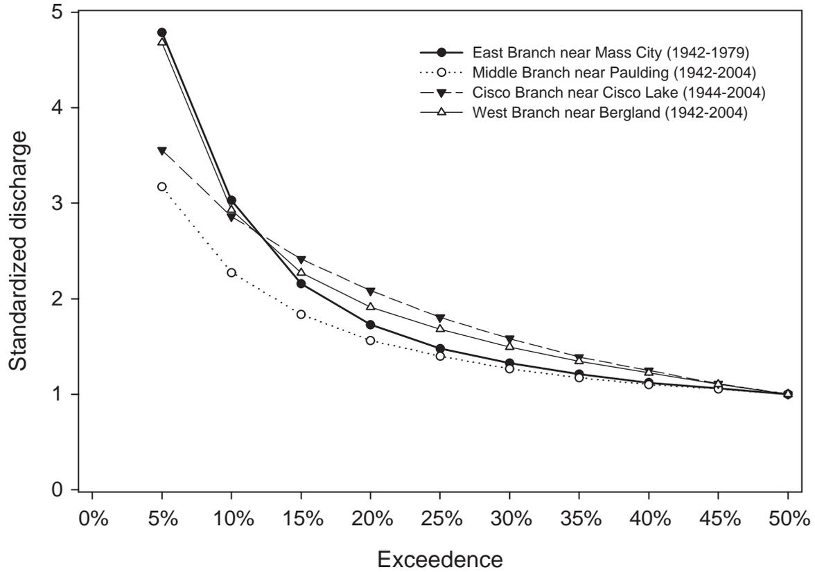
Figure 12.—Standardized high-flow duration curves for sites in the Ontonagon River watershed that are not affected by the Bond Falls diversion. Data from United States Geological Survey gauge stations for period of record.
