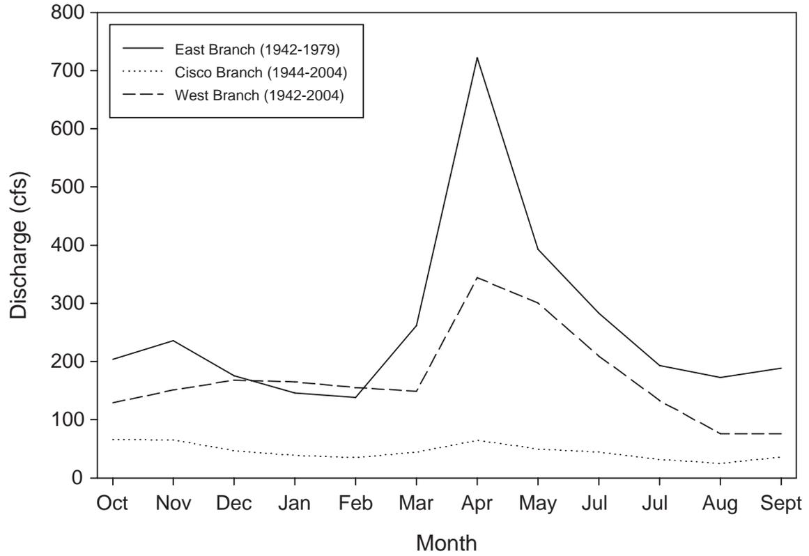
Figure 9.—Mean monthly discharge for the East, Cisco, and West branches of the Ontonagon River.
