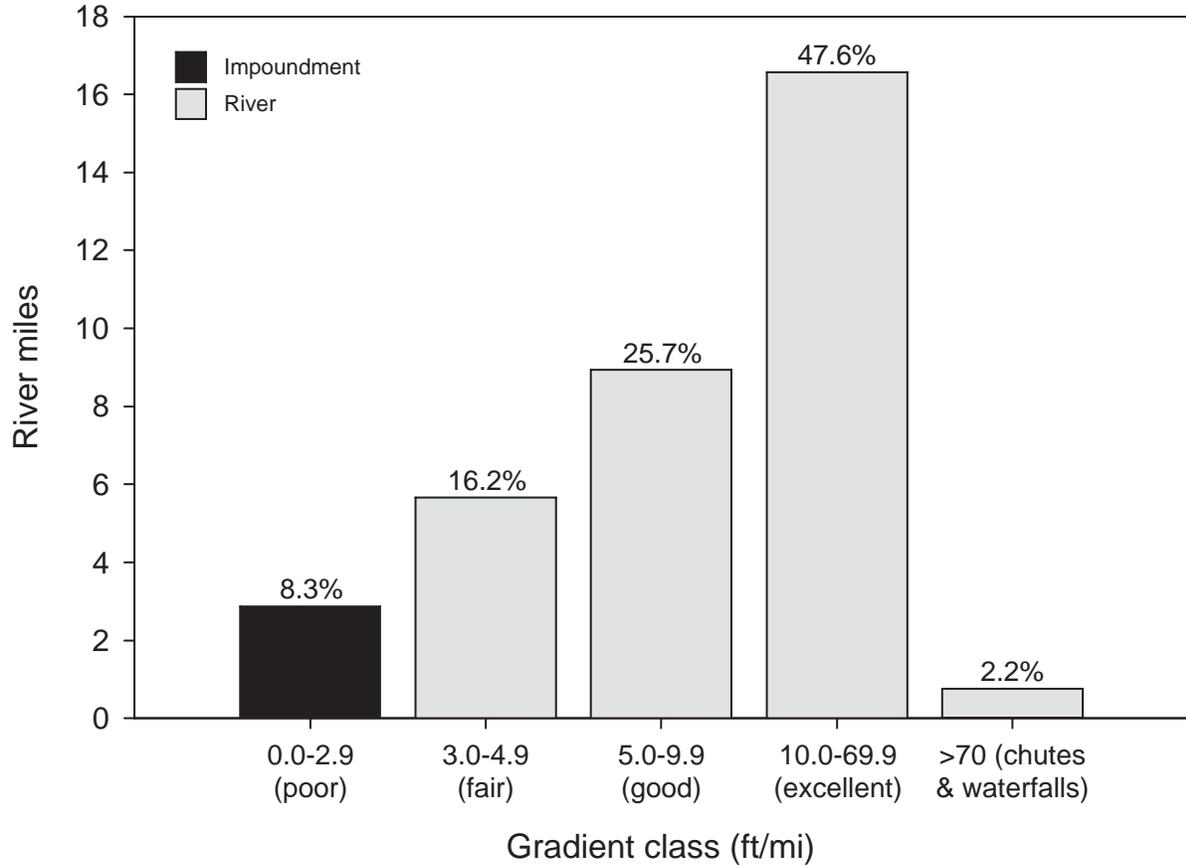
Figure 38.—Stream gradient distribution for the West Branch Ontonagon River. Fish habitat ranking in parentheses.
