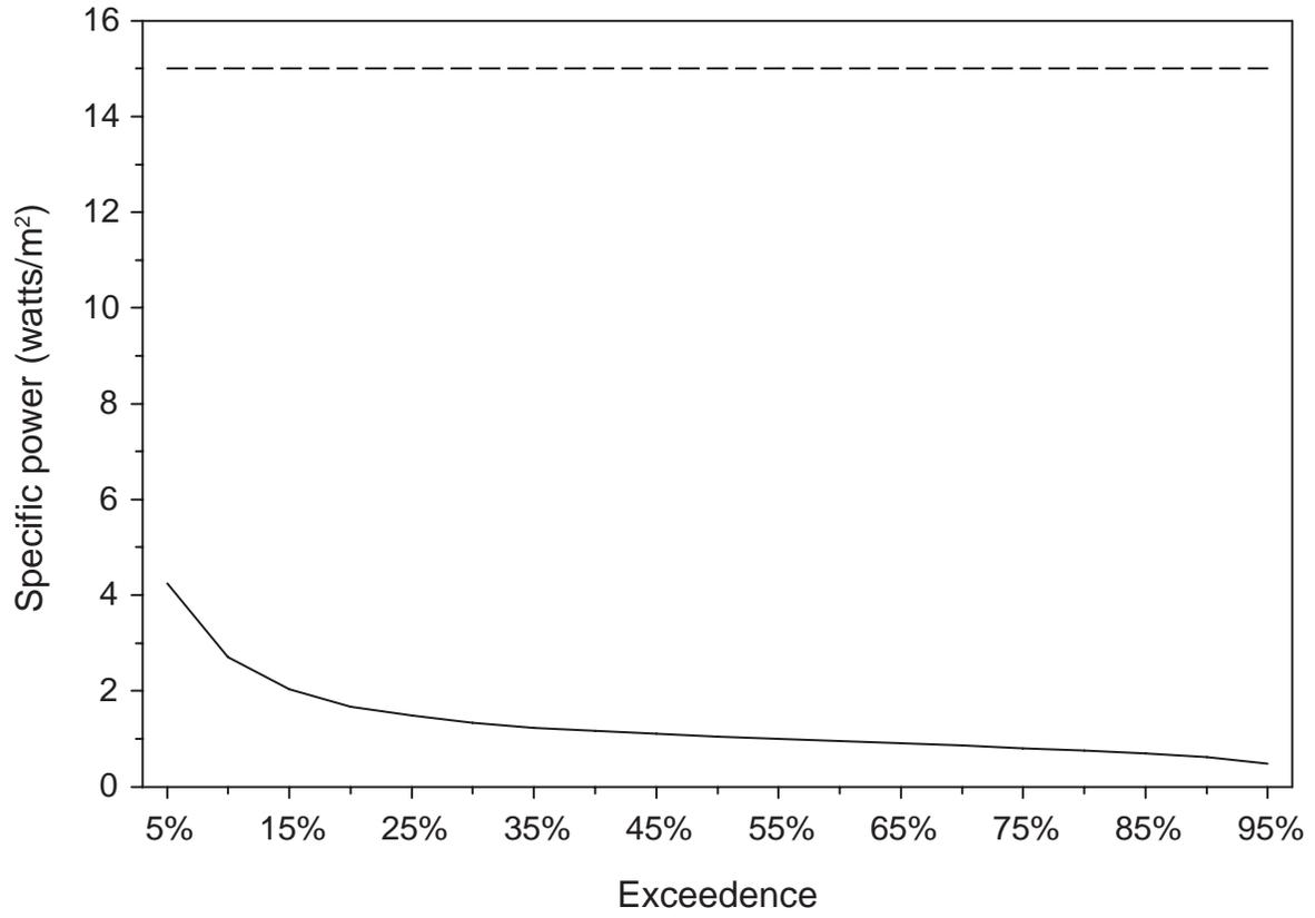
Figure 36.—Specific power for the South Branch Ontonagon River at Ewen.
