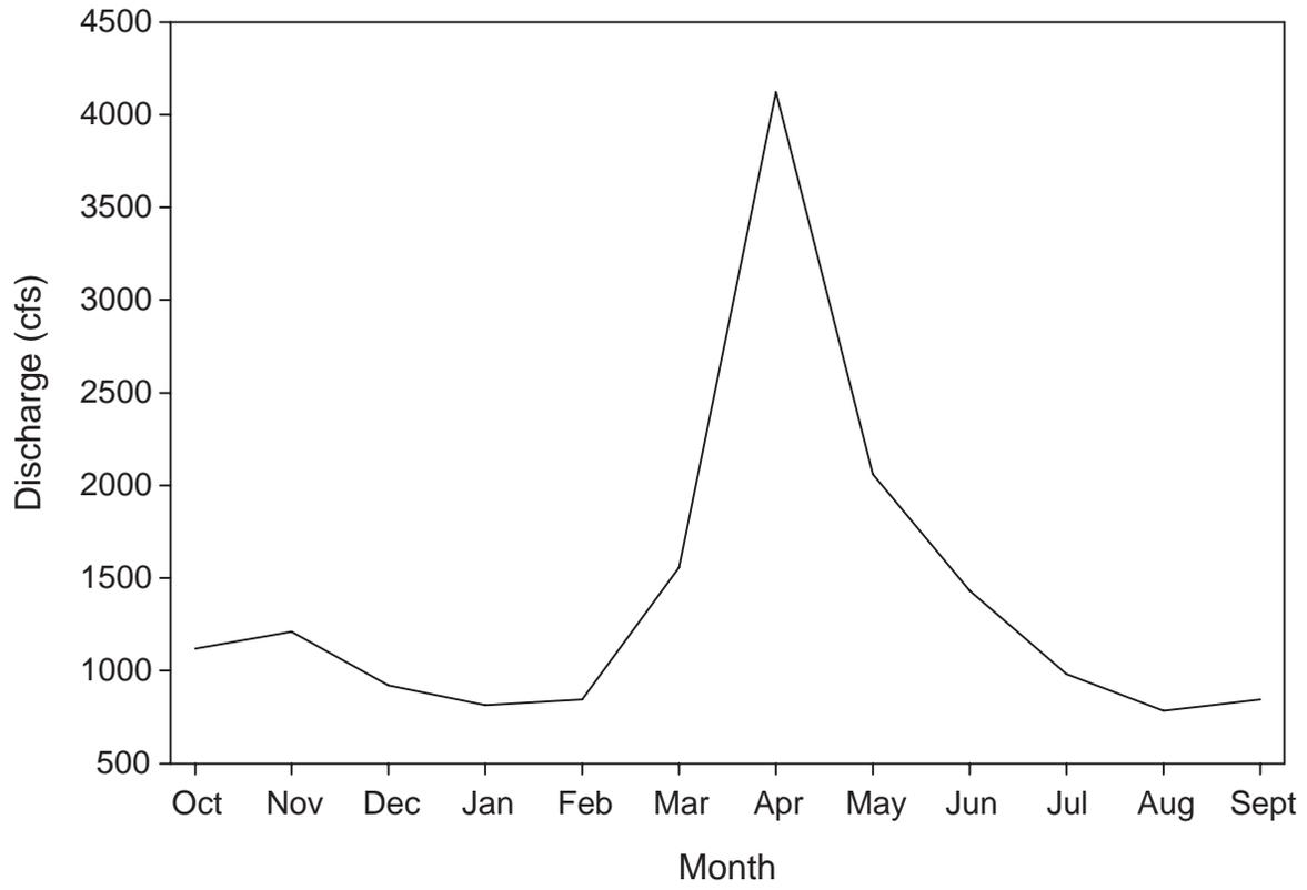
Figure 8.—Mean monthly discharge for the Ontonagon River near Rockland, 1942–2004.
