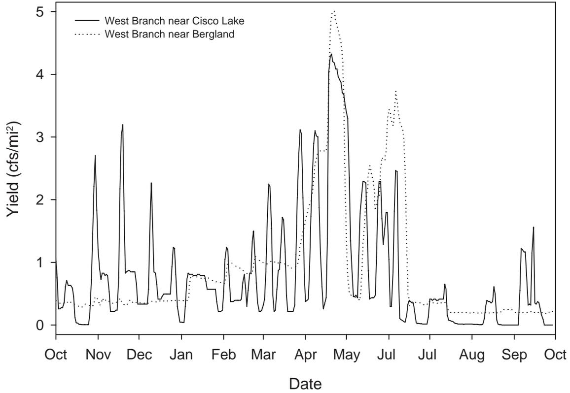
Figure 16.—Daily water yields for the Cisco Branch Ontonagon River and the West Branch Ontonagon River during October 2003 through September 2004. Data from United States Geological Survey.
