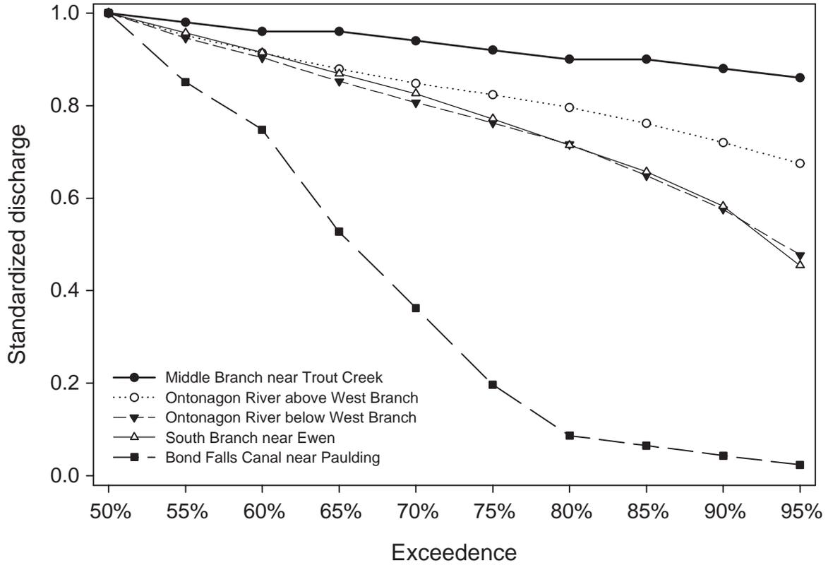
Figure 13.—Standardized low-flow duration curves for sites in the Ontonagon River watershed that are affected by the Bond Falls diversion. Data from United States Geological Survey gauge stations. Period of record was 1942–71 for the South Branch and 1942–2004 for the other four sites.
