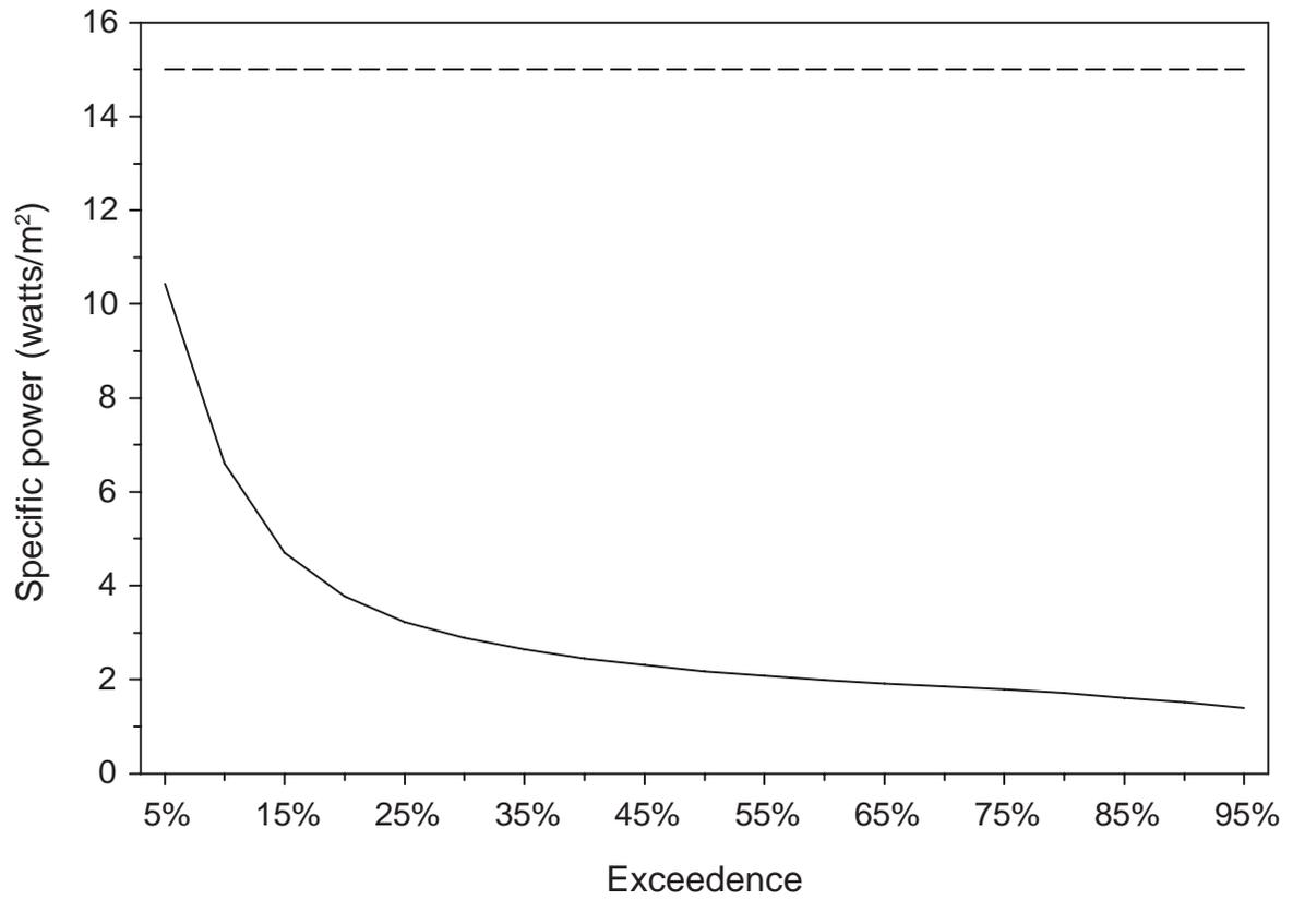
Figure 31.—Specific power for the East Branch Ontonagon River near Mass City.
