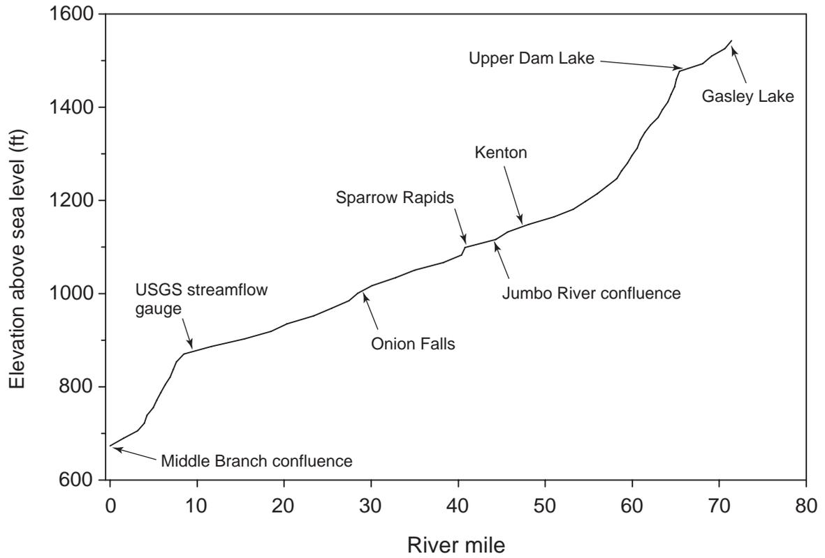
Figure 29.—Elevation changes by river mile for the East Branch Ontonagon River.
