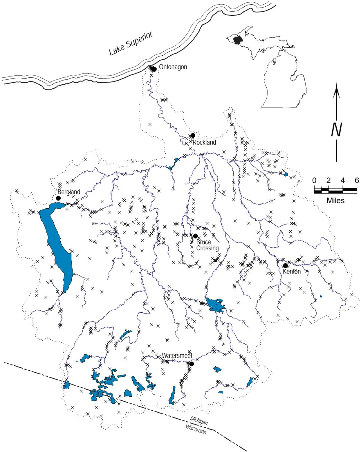
Figure 20.—Stream crossings in the Ontonagon River watershed (includes roads, railroads, and utilities). Stream crossing data derived from MIRIS Base Data (1998).
