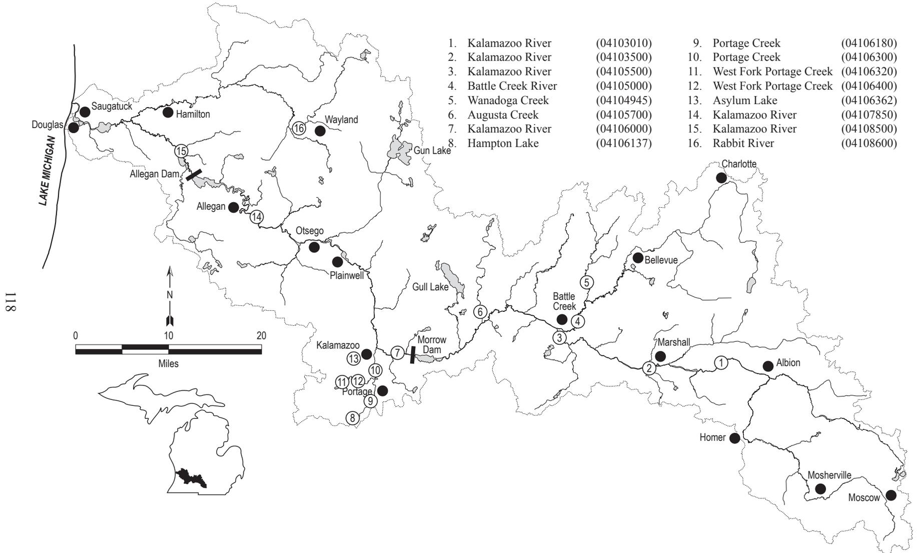
Figure 7.—Location of United States Geological Survey (USGS) continuous gauges in Kalamazoo River watershed. USGS identification number in parentheses.
