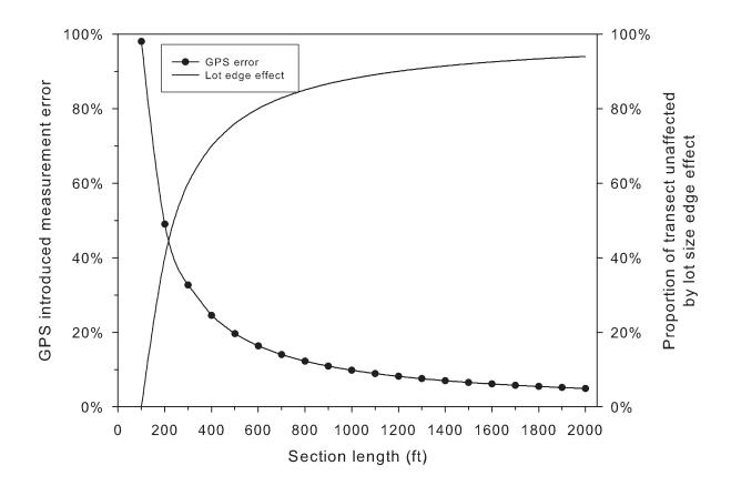
Figure 17.—Global positioning system (GPS) introduced error and percent of transect unaffected by lot width effect. For lot width evaluation, lot width was 60 ft.
