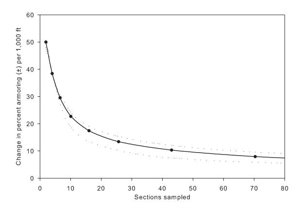
Figure 10.—Detectable change in mean shoreline armoring counts by sections sampled (1,000-ft transects) for selected Michigan large lakes. Sample size estimates were averaged across lakes for a given level of change and all three lakes were sampled. Estimates of precision are for  $\alpha$  = 0.05. Dotted lines represent minimum and maximum values from individual lakes.
