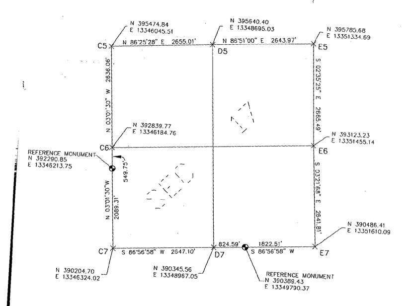
NOTE: DISTANCES ARE MEASURED AT GROUND AND COORDINATES ARE ON GRID
