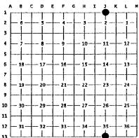
(J - 13) 1/4 Corner Common to Sections 35, T48N, R39W & Section 2, T47N, R39W.
