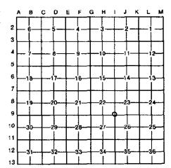
B. Description of corner evidence found and/or method applied in restoring or reestablishing corner: Southwest corner of Section 23 was found 2" bar bent over pipe which was set by Henning 1947, said corner in Pav't Box. All witnesses destroyed.
