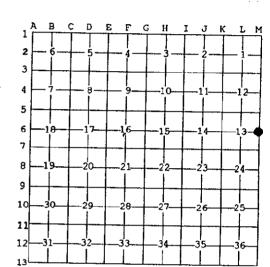
Description of corner evidence found and/or method applied in restoring or reestablishing corner: Fnd 1" Pipe with Department of Conservation 4" Brass Cap
